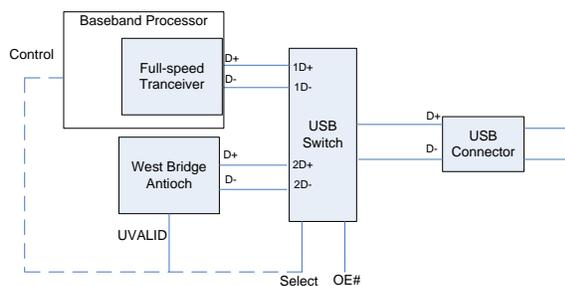
If the switch is SPST, the West Bridge Antioch device is connected at the output port of the switch and connected directly to the D+ and D- lines of the USB connector. The input port of the switch is connected to the transceiver of the baseband or applications processor. When the integrated transceiver is in use, the USB switch is enabled and West Bridge Antioch tristates its D+ and D- lines.
