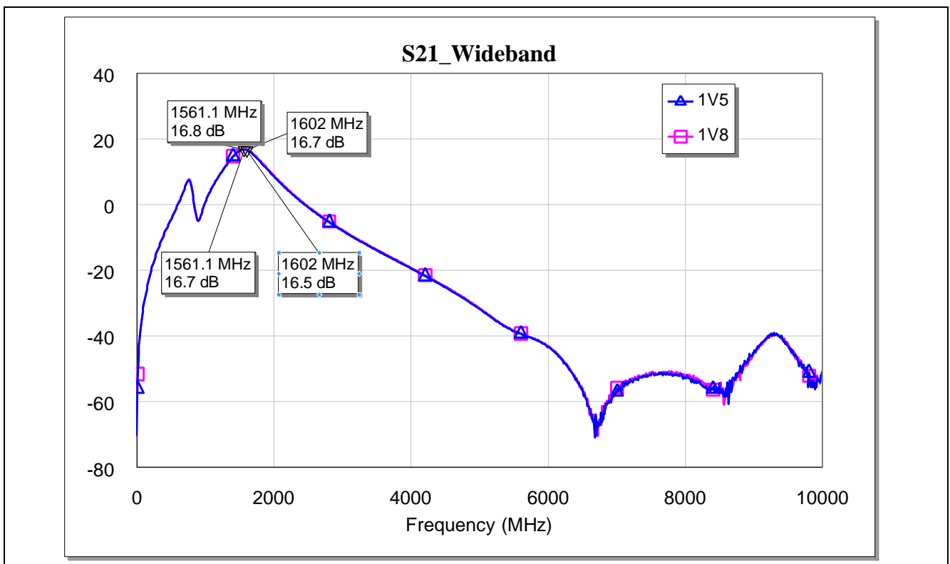
Figure 6 Wideband Gain of BGA524N6 as LNA for GNSS applications
