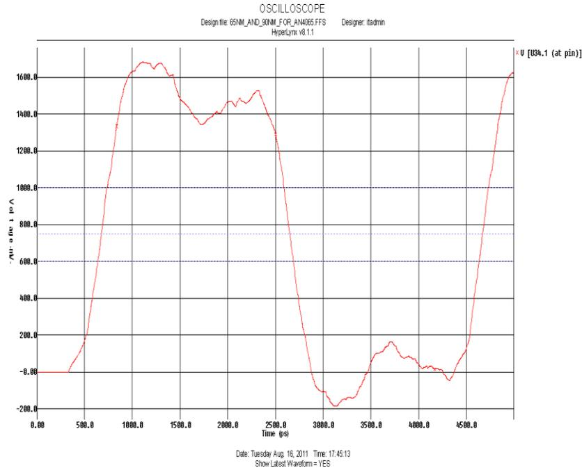
Figure 17. Eye Diagram for Source Impedance Matched Case
