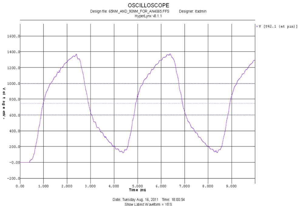
Figure 27 shows the eye diagram for the series resistor termination scheme shown in Figure 25. The eye width is 1.66 V, and the eye height is 931 mV.
