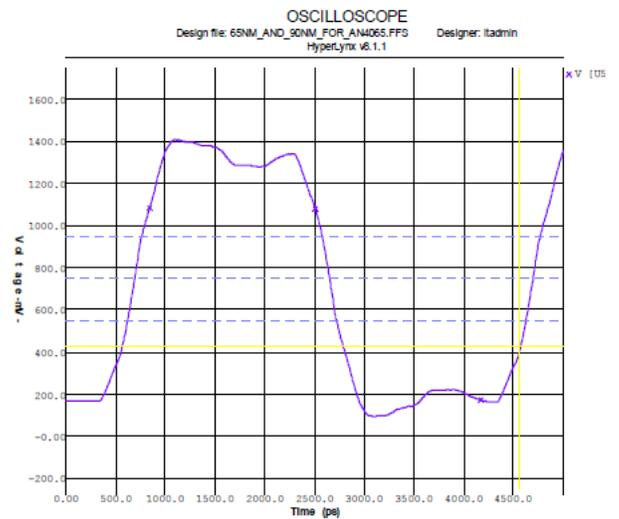
Figure 23. Simulation Result From Active Pull-Up Termination Scheme Using 50 Ω
