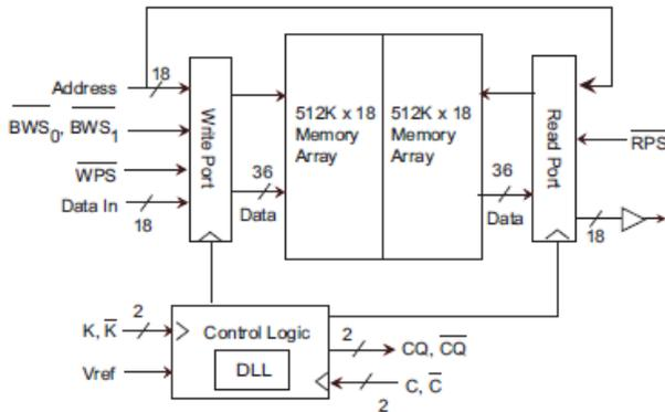
For the burst of four option, both the read and write address is provided on the rising edge of the K clock. The write data is provided with 1-clock cycle latency. For QDR-II, the read data is driven out after a 1.5-clock cycle latency, whereas for QDR-II+, the read data is driven out after 2.0 clock cycles or 2.5 clock cycles depending on the respective device option used.
