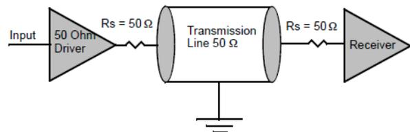
Figure 26. Using 50-Ω Series Resistances on Both Ends
