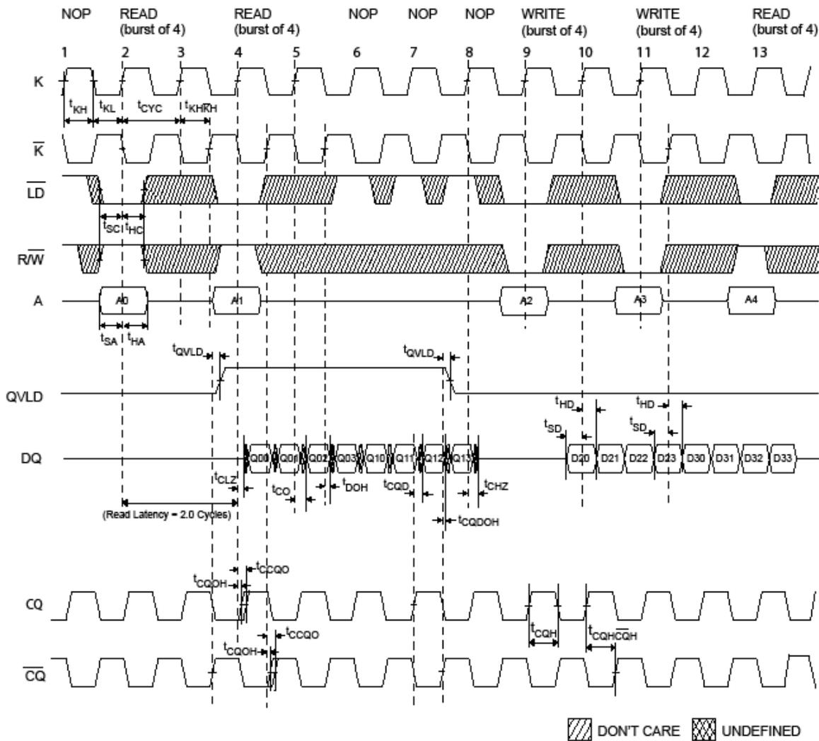
For detailed functional information with timing diagrams on QDR-II/II+ and DDR-II/II+, refer to the respective datasheets at [www.cypress.com](http://www.cypress.com).
