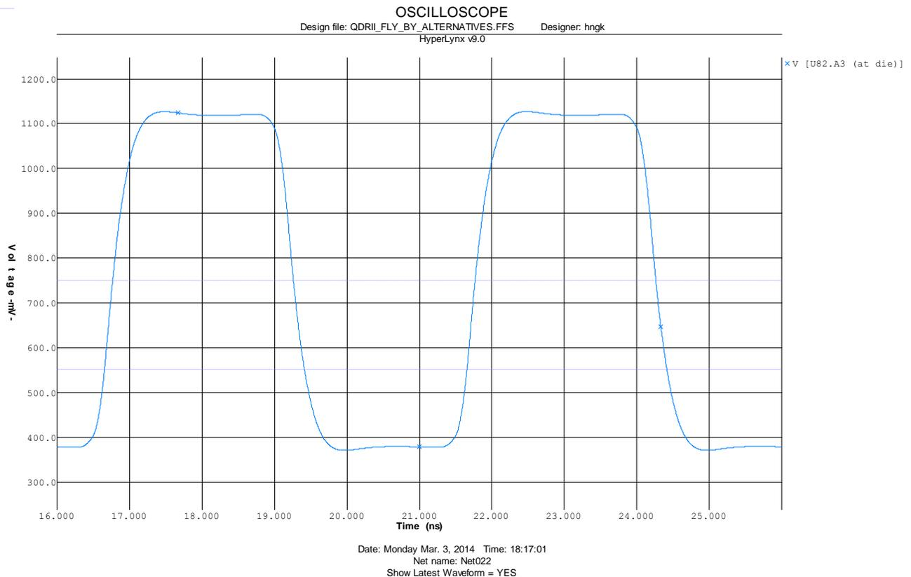
Figure 35 shows a more realistic fly-by topology where the distance between the receivers is 250 mils.
