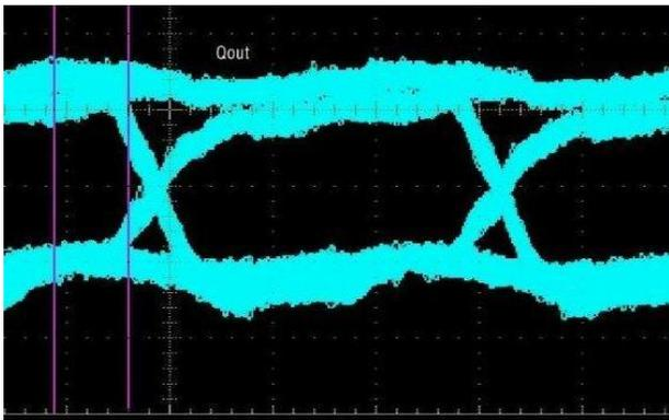
Figure 23 shows the simulation carried out from the topology shown in Figure 21 that has a single pull-up termination at the receiver end. Figure 24 shows the results from measurement of the board that has the same termination topology. The single pull-up receiver termination is the most recommended termination for the HSTL standard.
