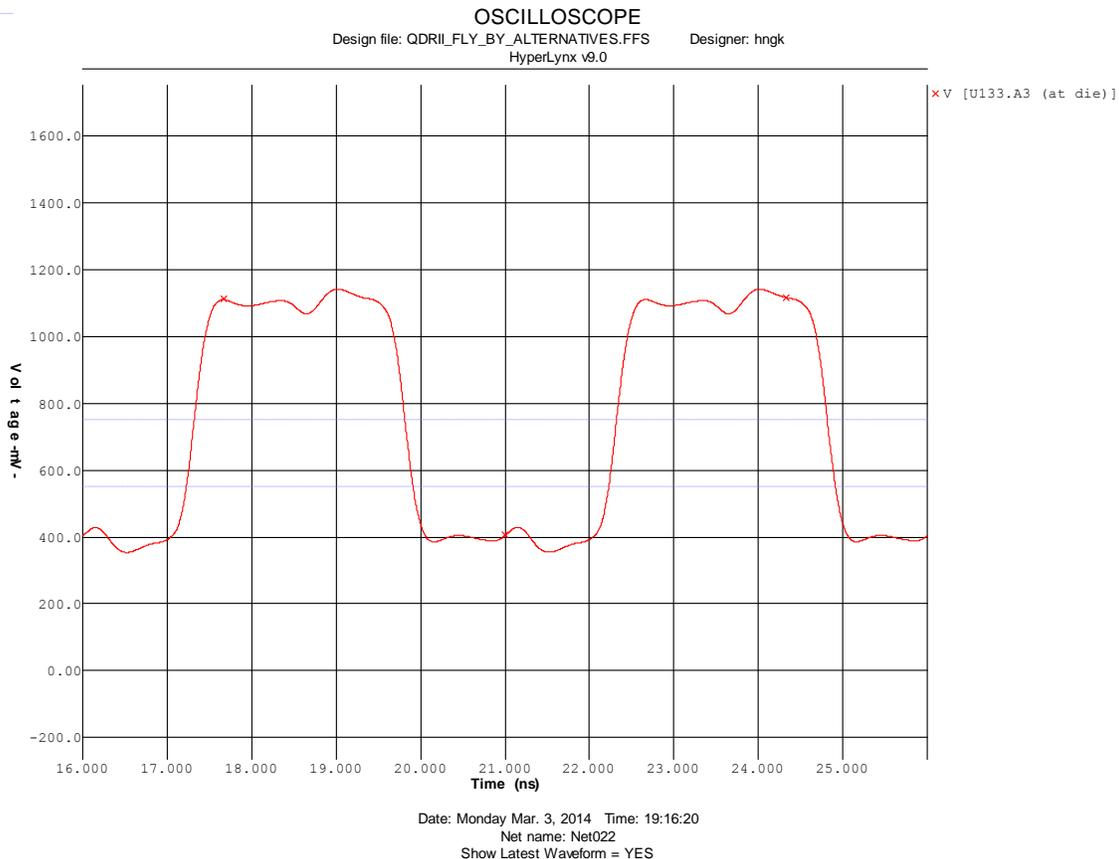
Both waveforms at the receiver inputs will be identical because the lengths and impedances are matched.
