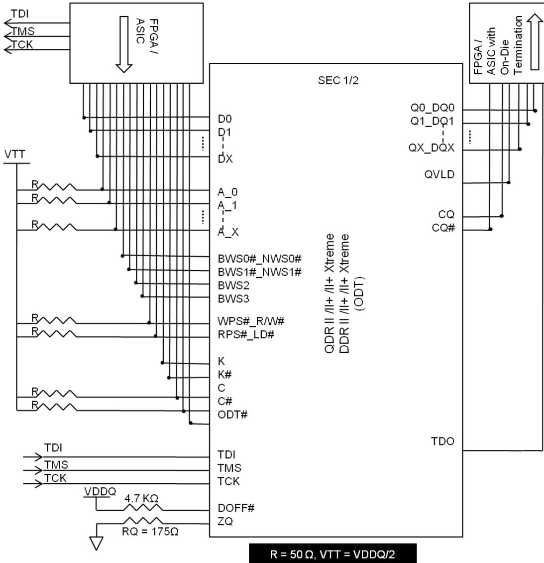
Figure 40. QDR II/II+/II+Xtreme-DDR II/II+/II+Xtreme (Supply Pins) Reference Schematic
