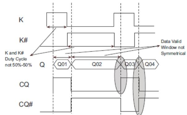
Refer to the [Clocking Strategy 1: Using Input Clock K/K#](#), [Clocking Strategy 2: Using Input Clocks K/K#, C/C#](#), and [Clocking Strategy 3: Using Echo Clocks CQ and CQ#](#) sections to get more details on when and how to select the clock pair that can be used for latching data at the receiving controller (ASIC/FPGA).
