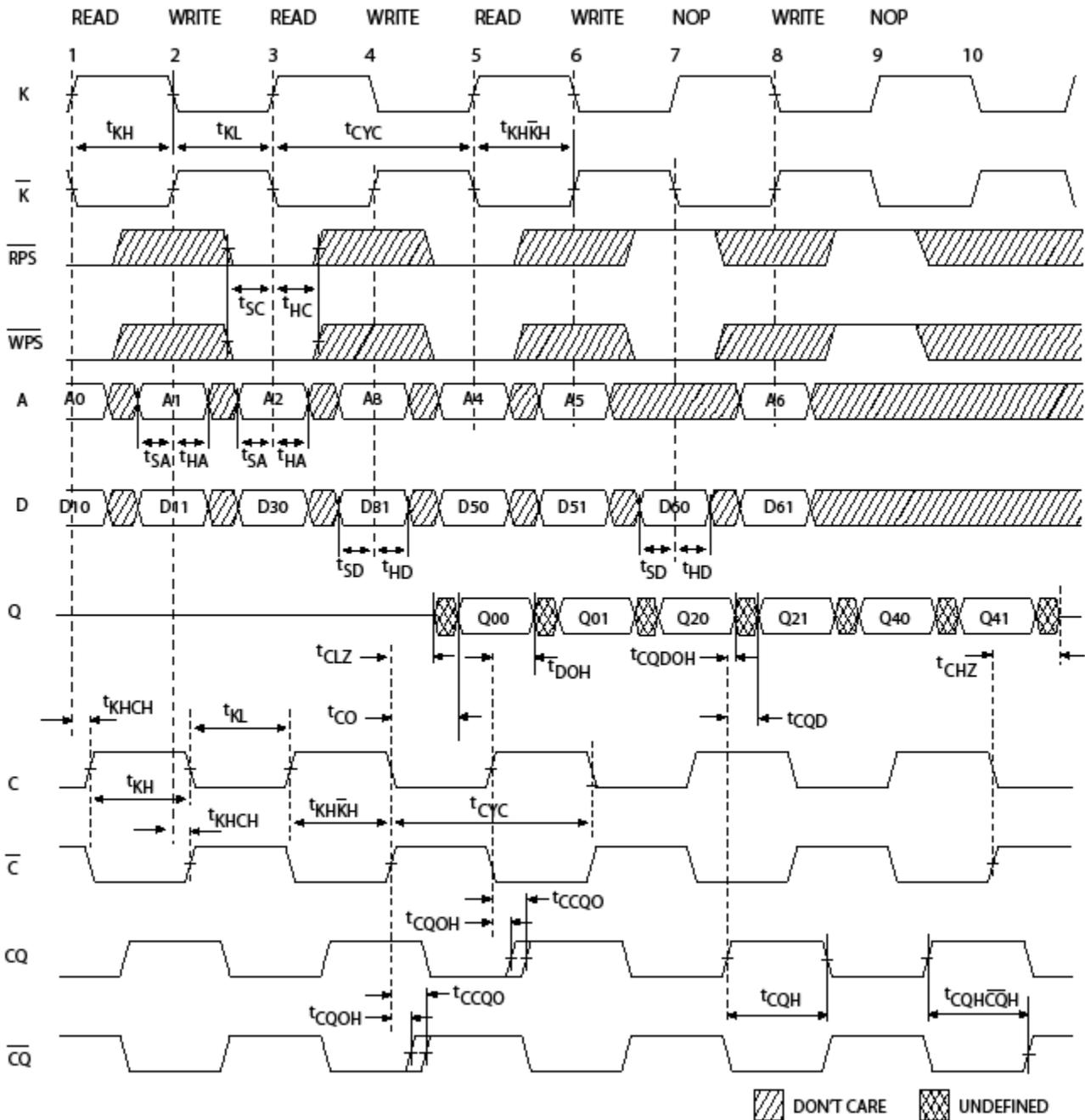
Figure 5. QDR-II/II+ Burst of Four Timing Showing Latency of Two
