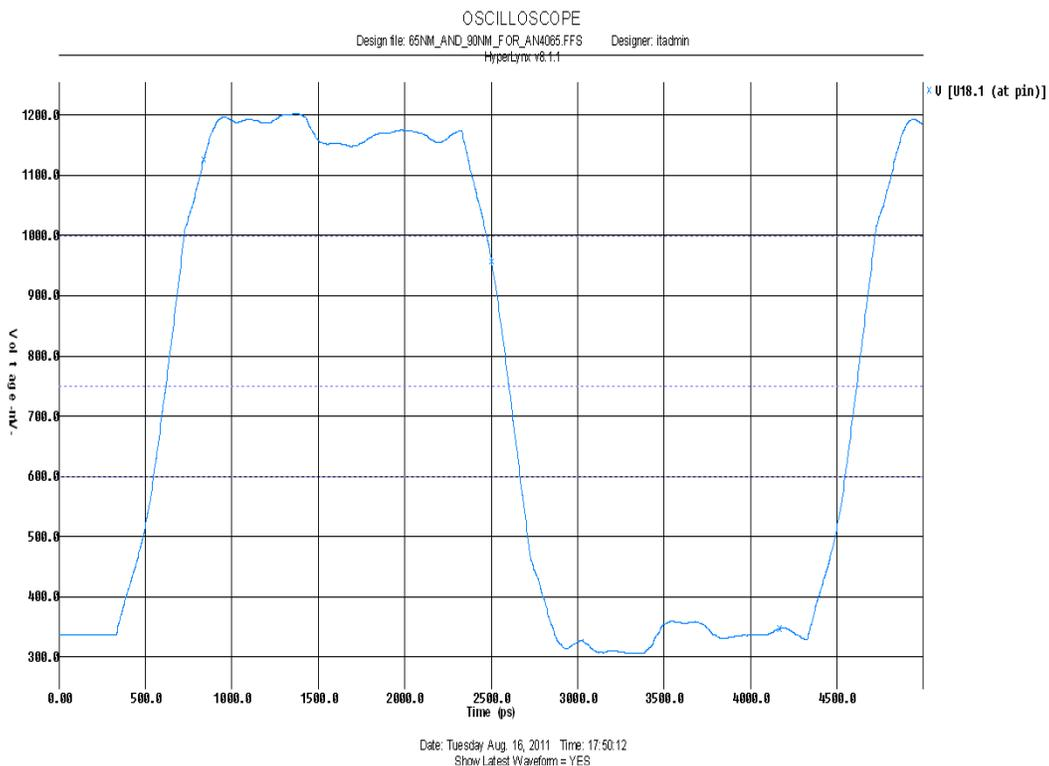
Figure 20. Eye Diagram for R1 = 50 Ω Active Pull-Up Termination Case
