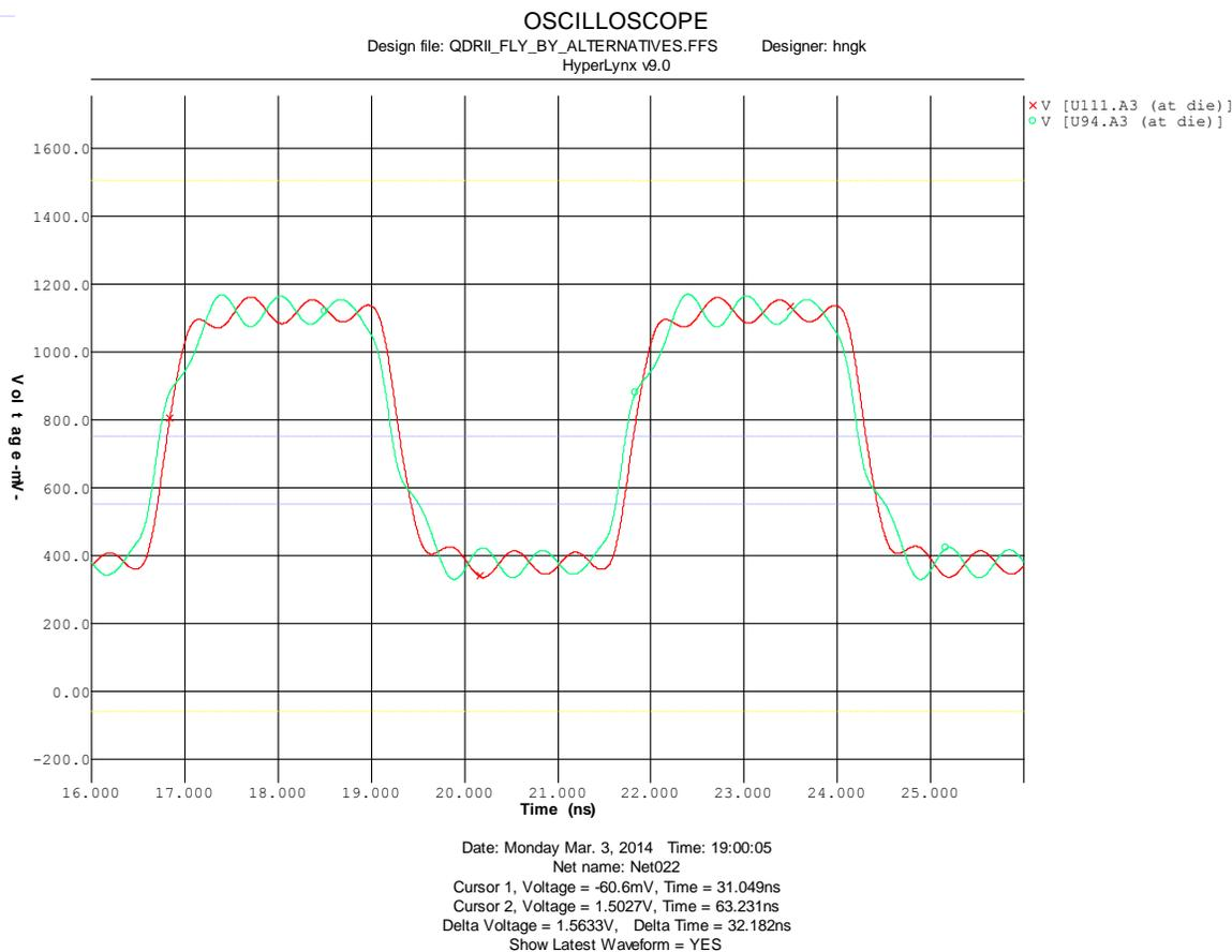
In general, using more memories (receivers) to extend the topology shown in [Figure 35](#) will cause waveform degradation unless the distances are reduced with more receivers.
