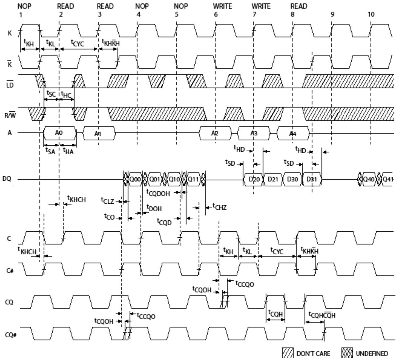
For the burst of four option, the read or write address is provided on every other rising edge of the K clock. The write data is provided with a 1-clock cycle latency. DDR-II read data is driven out after a 1.5-clock cycle latency whereas DDR-II+ read data is driven out after 2.0 clock cycles or 2.5 clock cycles depending on the respective device option used.
