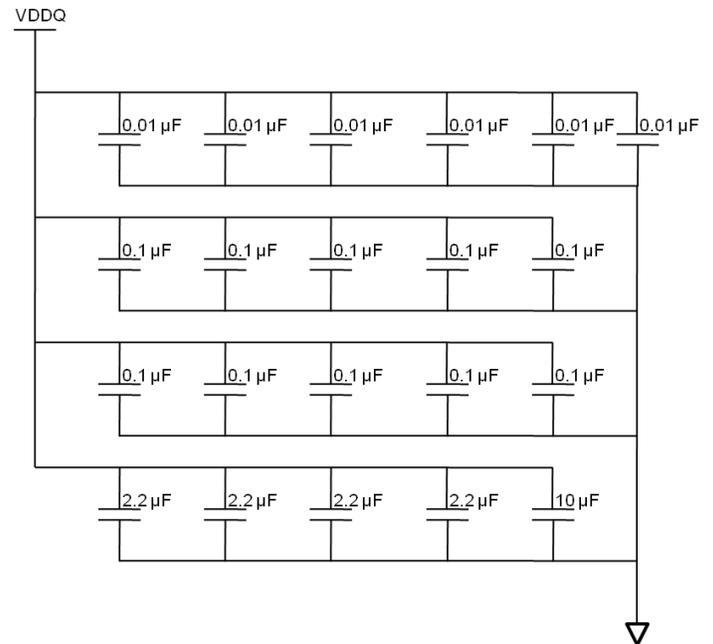
Figure 43. Decoupling Capacitor Recommendation for  $V_{TT}$
