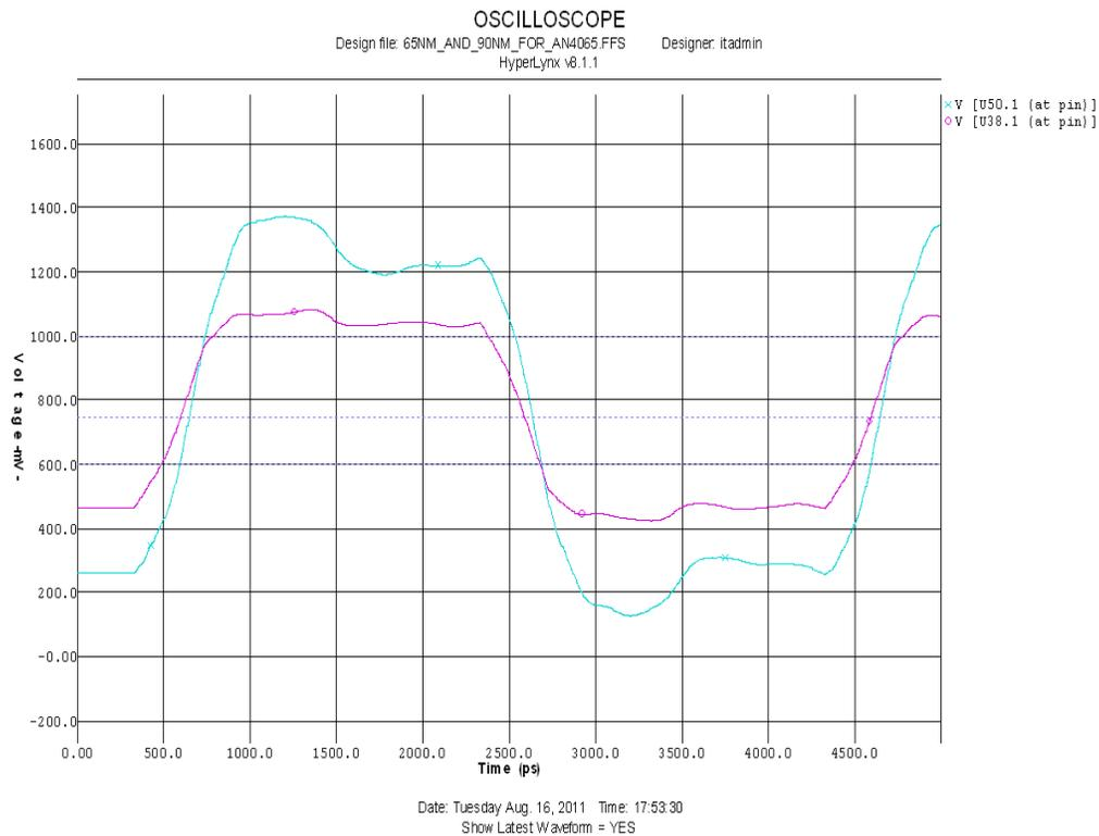
As seen in Figure 30, the voltage swing for the Active Pull-up termination using 50 Ω is from 425 mV to 1.1 V, and for the Active Pull-up termination of 150 Ω is from 130 mV to 1.38 V.
