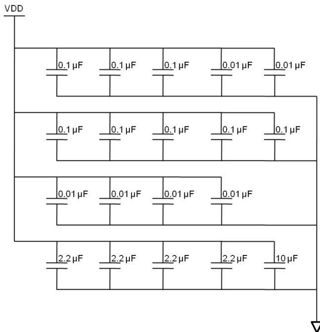
Figure 42. Decoupling Capacitor Recommendation for  $V_{DDQ}$
