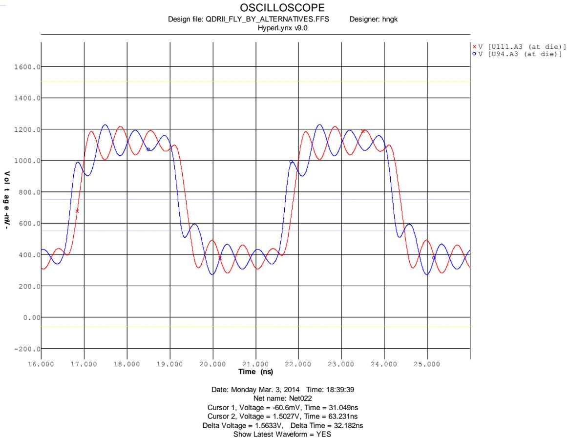
Figure 37. Simulation Results for Fly-By Topology: 150-mil Separation Between Receivers
