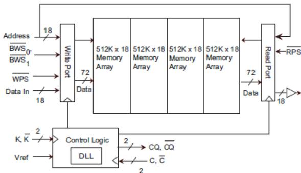
Figure 3. QDR-II+ Burst of Four Device (2 M x 18)
