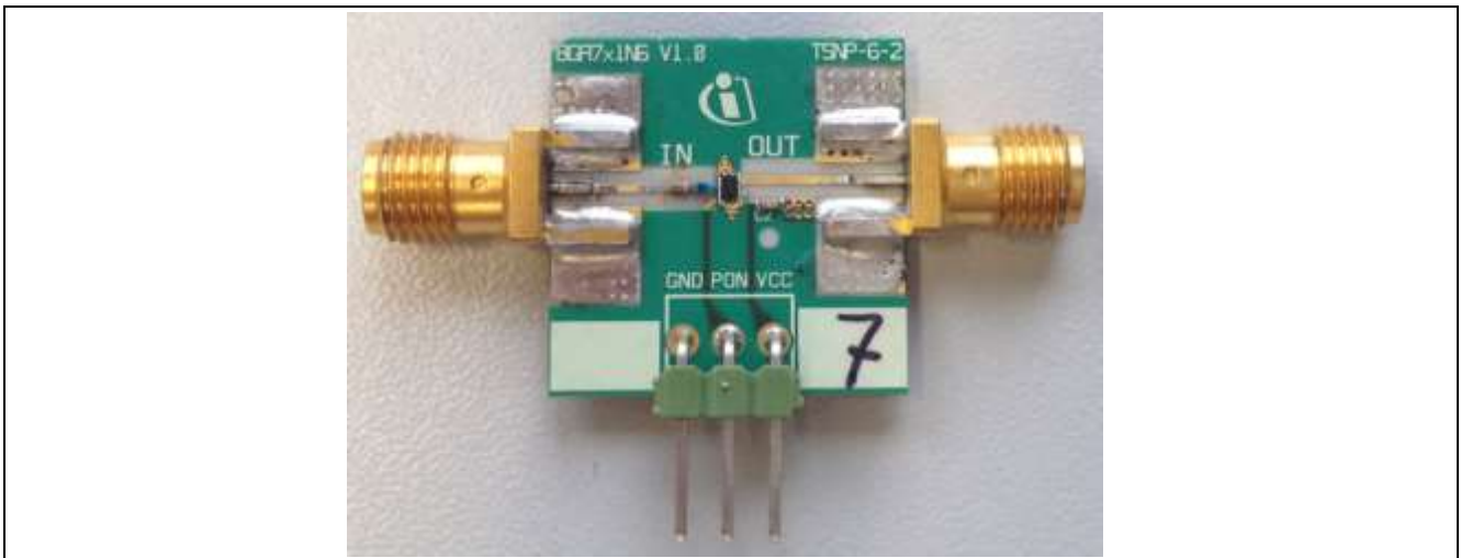
Figure 29 Photo of Evaluation Board (overview)
