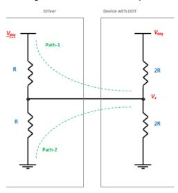
Figure 2. ODT Power Consumption
