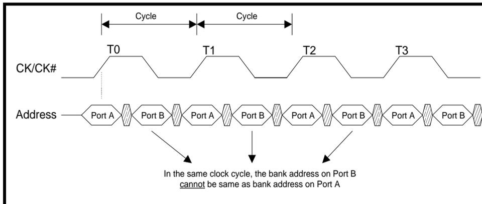
Figure 10. QDR-IV HP SRAM – Write/Read Operation
