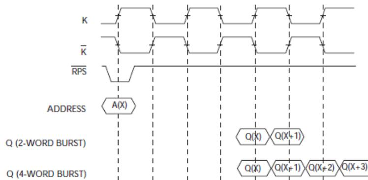
Output data is coherent. If a Read and a Write cycle are initiated during the same clock cycle (at  $K$  rising edge),  $\overline{RPS}$  and  $\overline{WPS}$  are both LOW. A Read is requested from address 1; address 1 is provided. At  $\bar{K}$  rising edge, address 2 is provided for the Write. In this example, addresses 1 and 2 are the same. The Read data provided is the same data presented for the Write to address 2.
