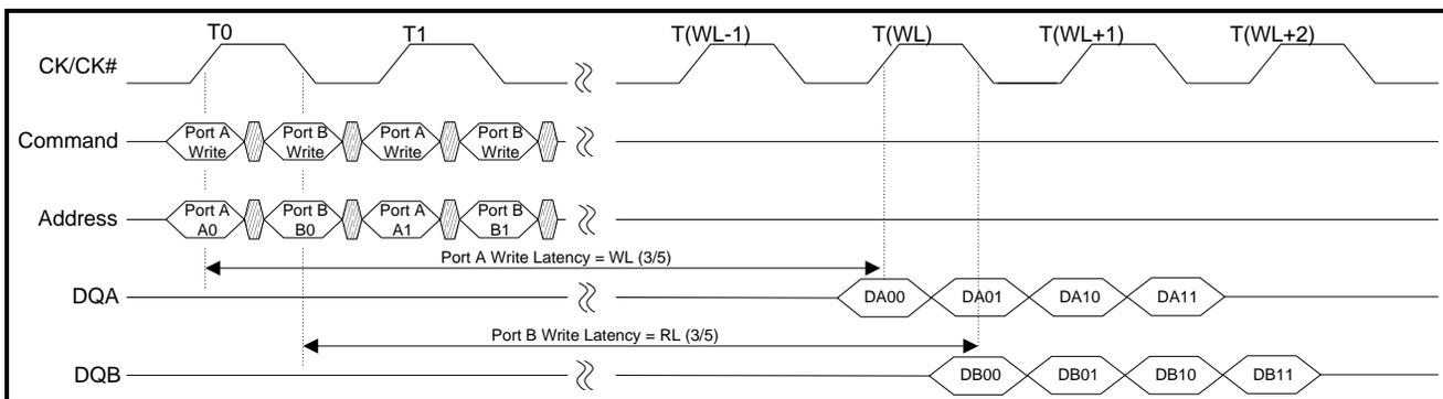
The QDR-IV XP SRAM is designed with eight internal banks. The lower three address pins (A2, A1, and A0) select the bank that will be accessed during a read or write operation.
