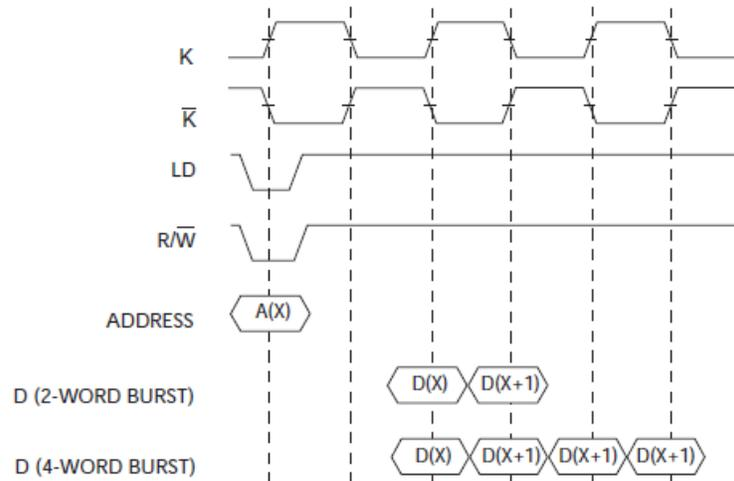
Figure 6. DDR-II Read Cycle
