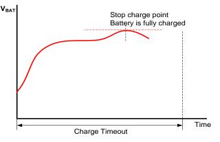
The charge stage should be limited by a timeout that extends for approximately 120 to 150 percent of the estimated time required to charge NiCd/NiMH batteries with expected maximal capacity.
