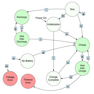
Figure 5. Charger State Diagram
