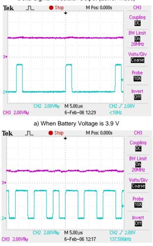
Figure 3. Integrator Output (Upper Trace) and Delta-Sigma Modulator Output (Lower Trace)
