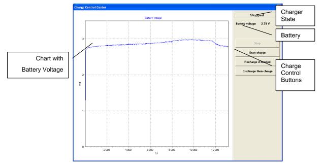
Figure 6. Charger Monitoring Software
