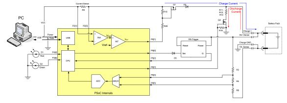
Figure 7. Charger Structure with Linear Regulator
