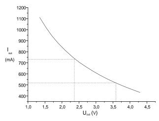
For the linear regulator, the current is constant and does not exceed 0.5 A. So when a switching regulator is used to charge two batteries (2.6 V in a charged state), the charge current is significantly greater than the charge current when a linear current source is used. For three batteries with 3.9 V in a charged state, the charge current is about the same for both kinds of regulators. For deeply discharged batteries (2.4 V), the charge current is greater.
