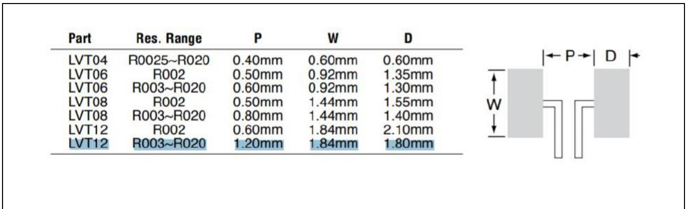
Figure 12 Typical SMD resistor packages and land patterns
