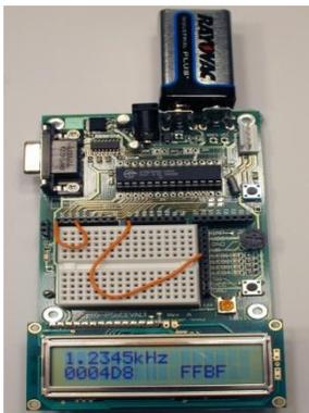
You might notice that the two resistors have been removed. Also, the two capacitors and a crystal have been added.
