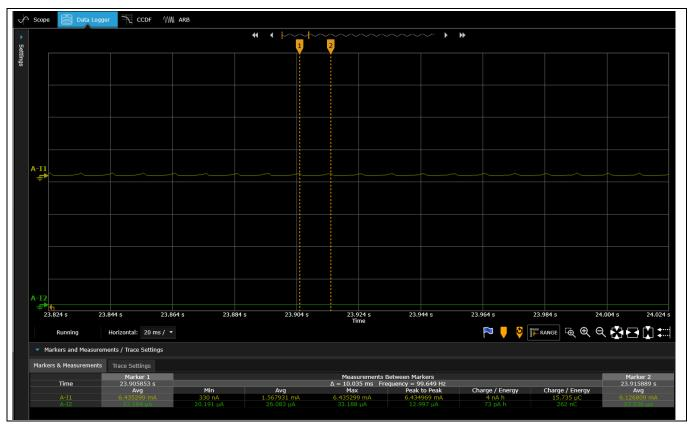
Figure 36 Current consumption with connection interval of 10 ms
