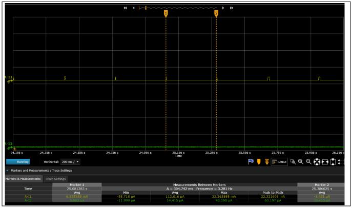
Figure 26 CY8CKIT-062S-43012 power consumption (associated, DTIM = 3, 2.4 GHz)
