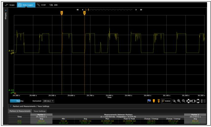
Figure 40 Current consumption during high-duty scanning
