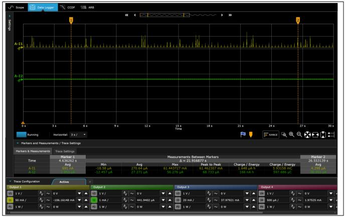
Figure 31 CY8CKIT-062S-43012 power consumption during ping activity
