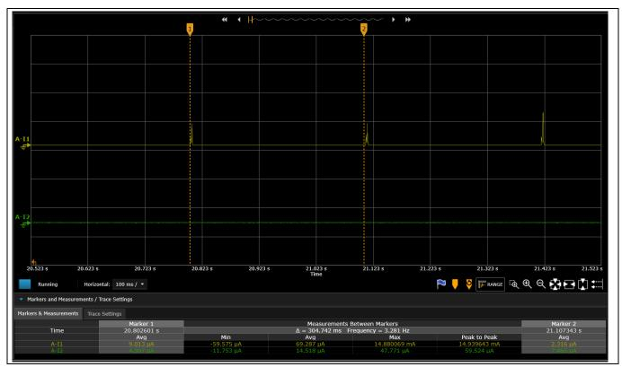
Figure 27 CY8CKIT-062S-43012 power consumption (associated, DTIM = 3, 5 GHz)
