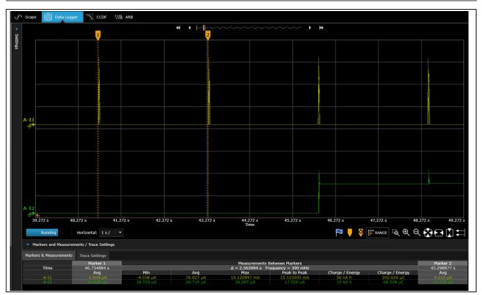
Figure 41 Current consumption during low-duty scanning
