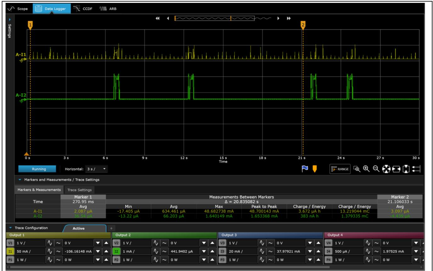
**Figure 32** CY8CKIT-062S-43012 power consumption during ping activity
