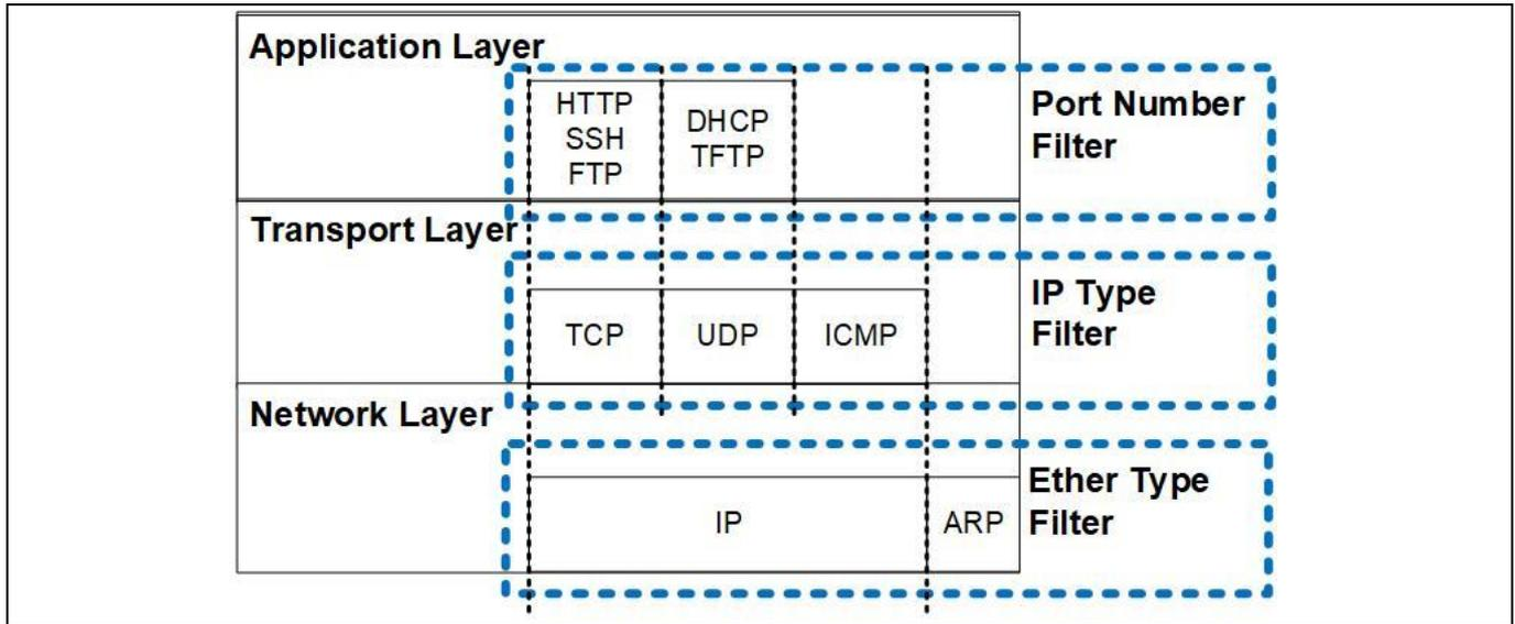
Figure 7 Packet filters
