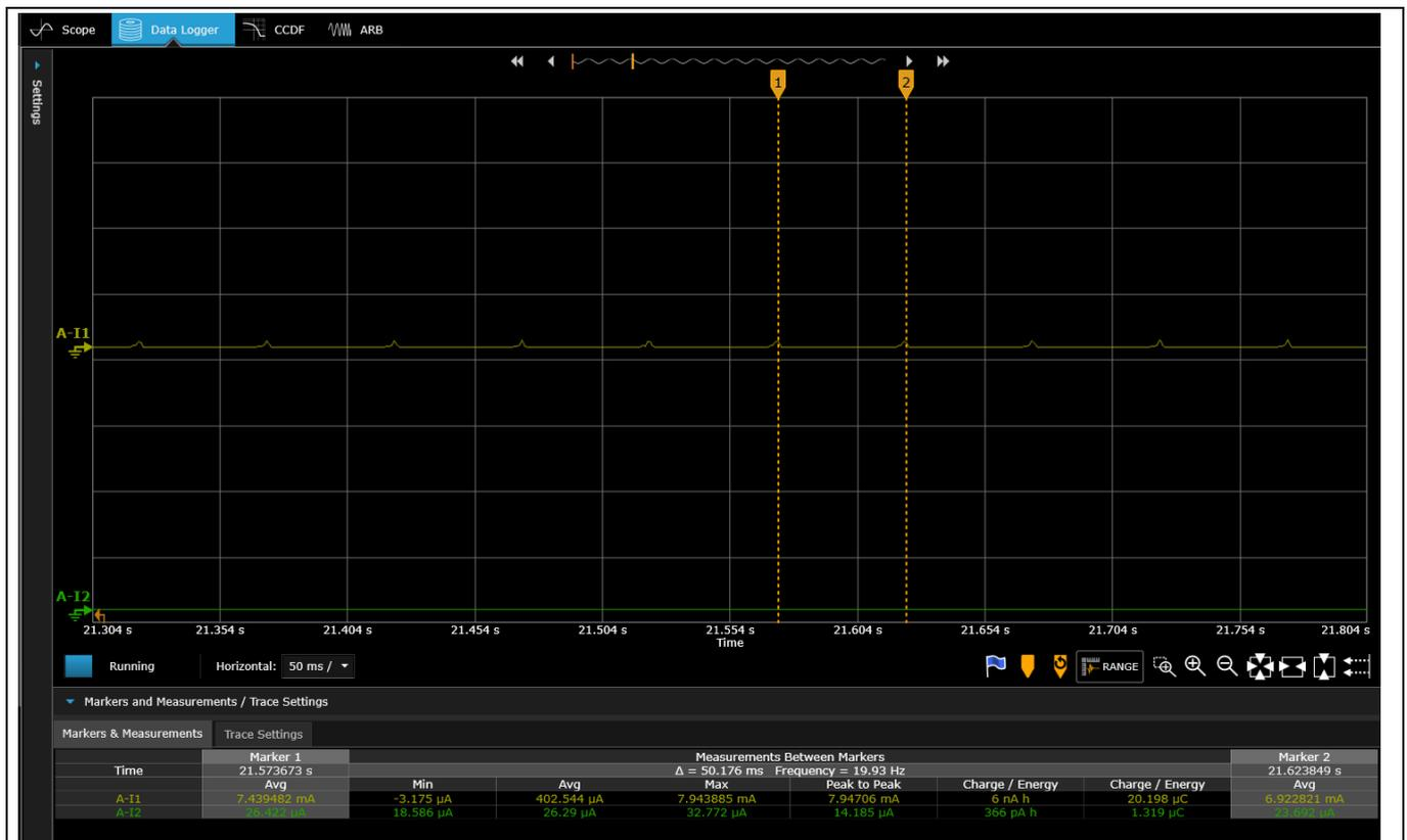
**Figure 37** Current consumption with connection interval of 50 ms
