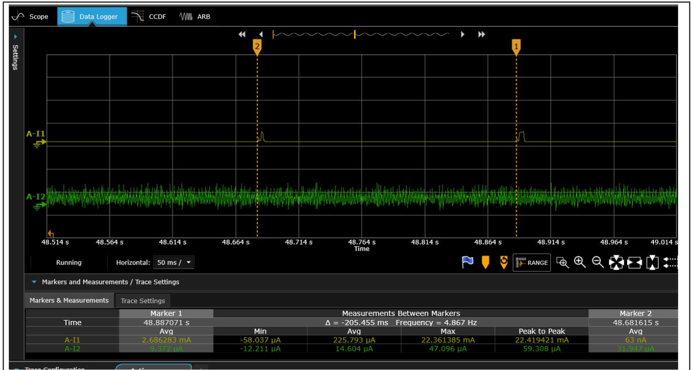
Figure 24 CY8CKIT-062S-43012 power consumption (associated, DTIM = 2, 2.4 GHz)
