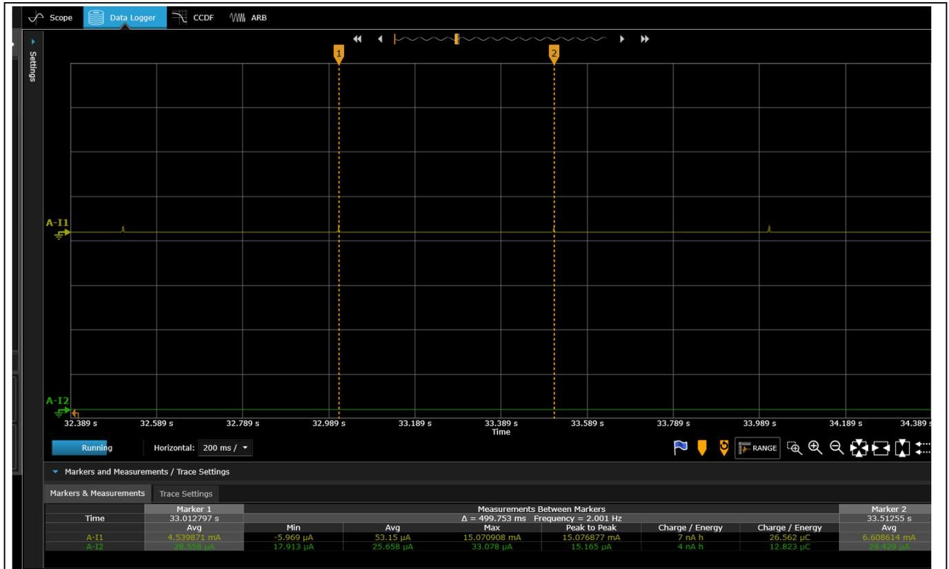
**Figure 38** Current consumption with connection interval of 500 ms
