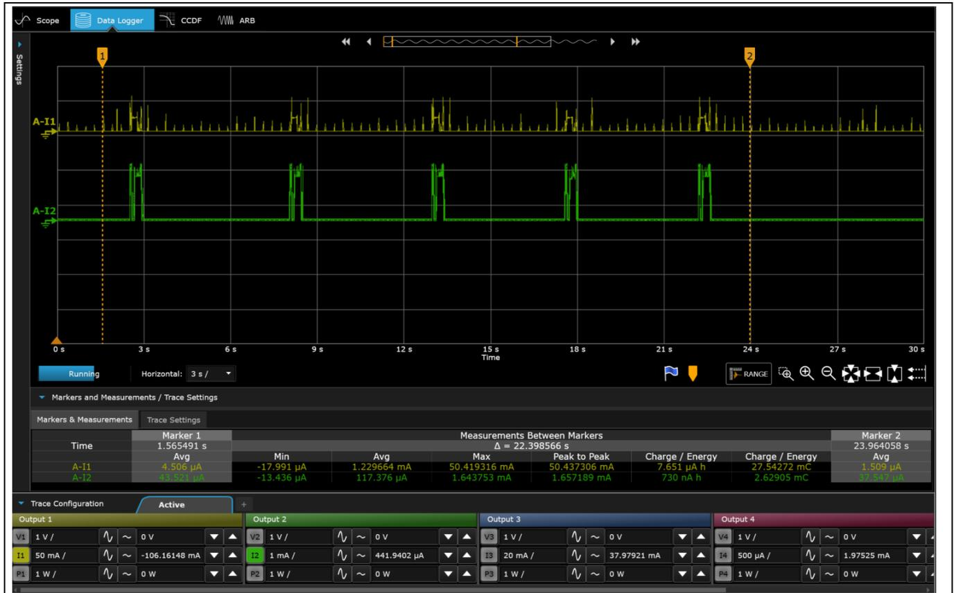
**Figure 33** CY8CKIT-062S-43012 power consumption during ping activity
