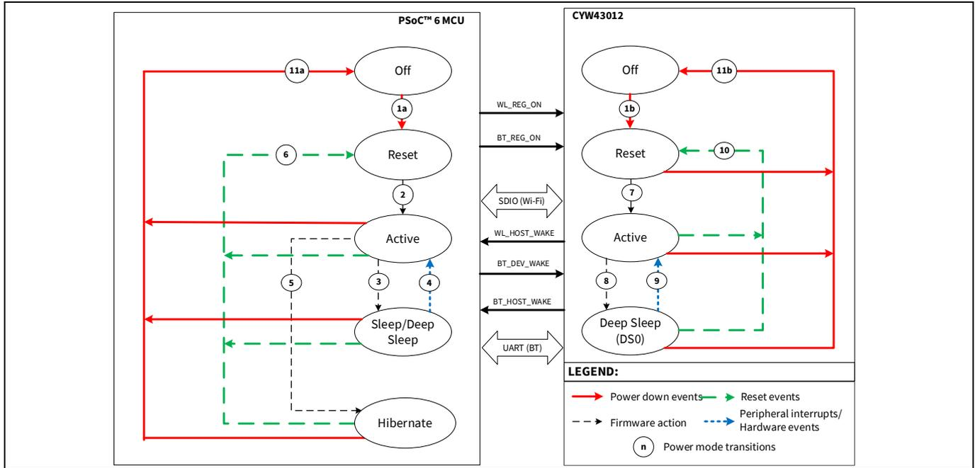
Figure 1 Simplified power mode transitions in “PSoC™ 6 MCU<sup>a</sup> + AIROC™ CYW43012 Wi-Fi & Bluetooth® combo chip” design
