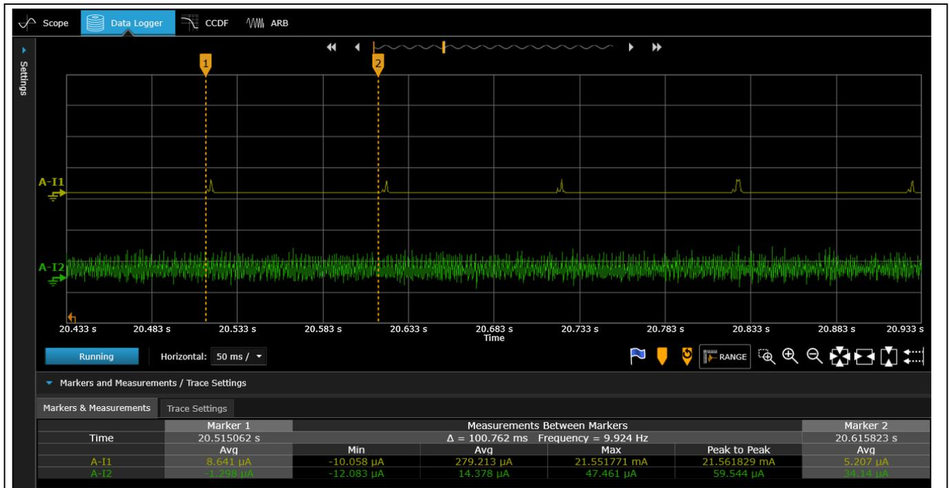
Figure 23 CY8CKIT-062S-43012 power consumption (associated, DTIM = 1, 5 GHz)
