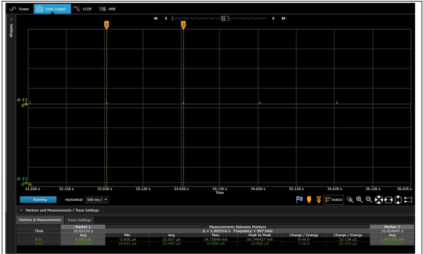
**Figure 39** Current consumption with connection interval of 1000 ms
