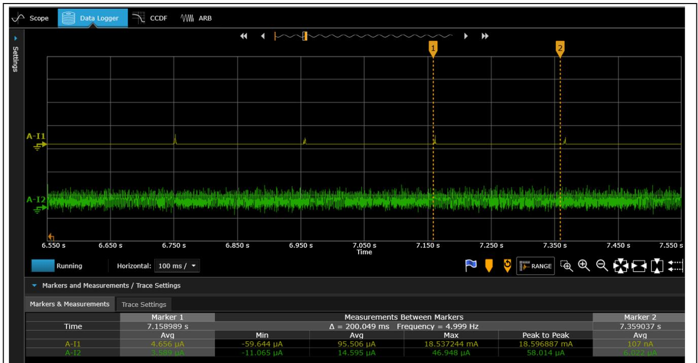
Figure 25 CY8CKIT-062S-43012 power consumption (associated, DTIM = 2, 5 GHz)
