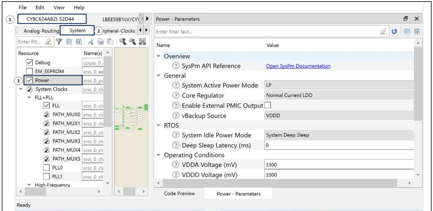
**Figure 13** PSoC™ 6 MCU LPA configurations in *design.modus*
