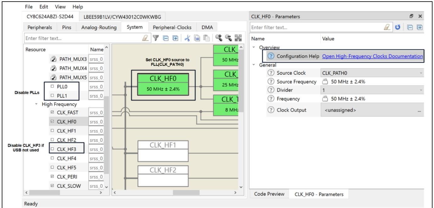
Figure 17 CY8CKIT-062S2-43012 clock setup for low power
