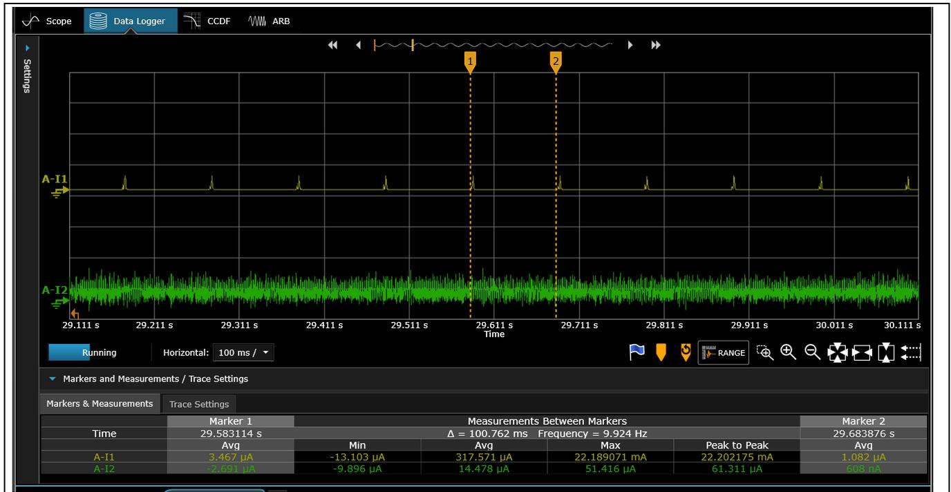
Figure 22 CY8CKIT-062S-43012 power consumption (associated, DTIM = 1, 2.4 GHz)
