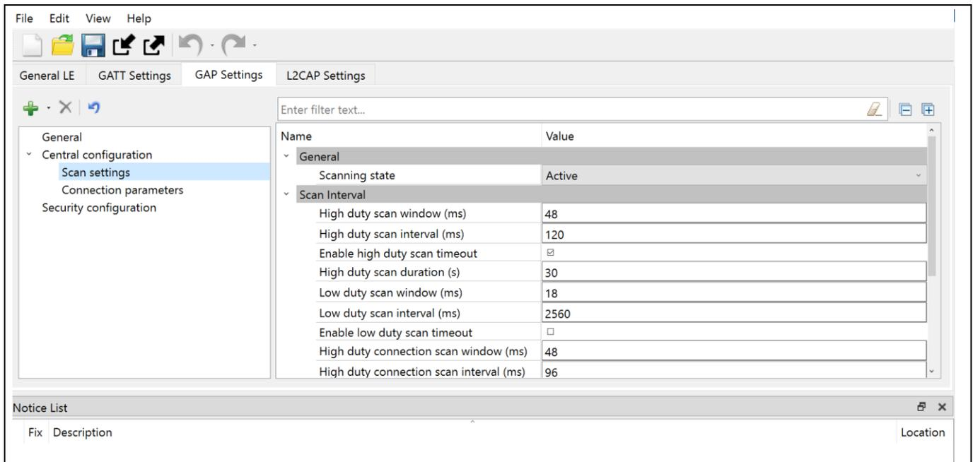
Figure 12 Scan settings in Bluetooth® Configurator
