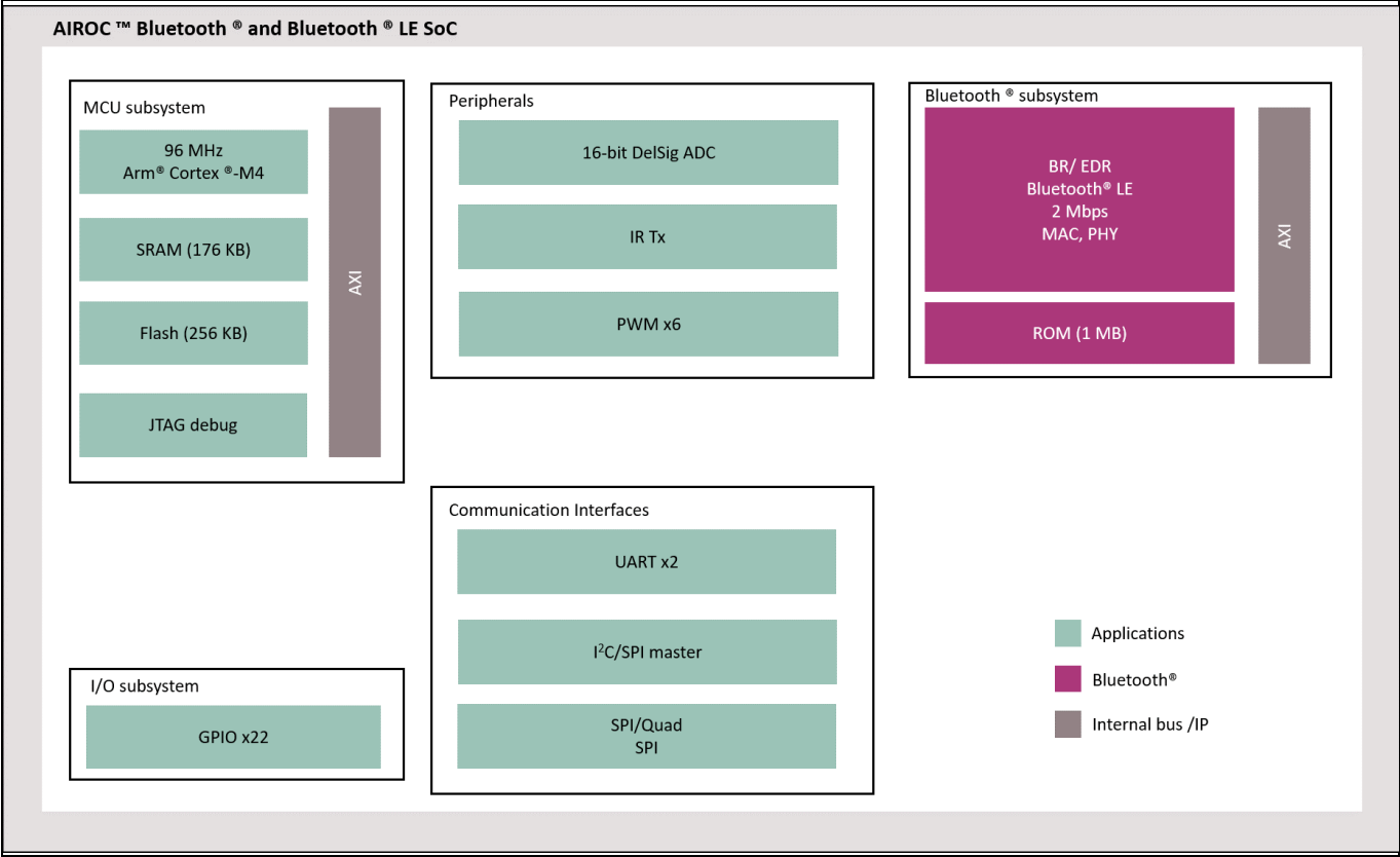
Figure 1 Block diagram of CYW20819/CYW20820 Bluetooth® SoC
