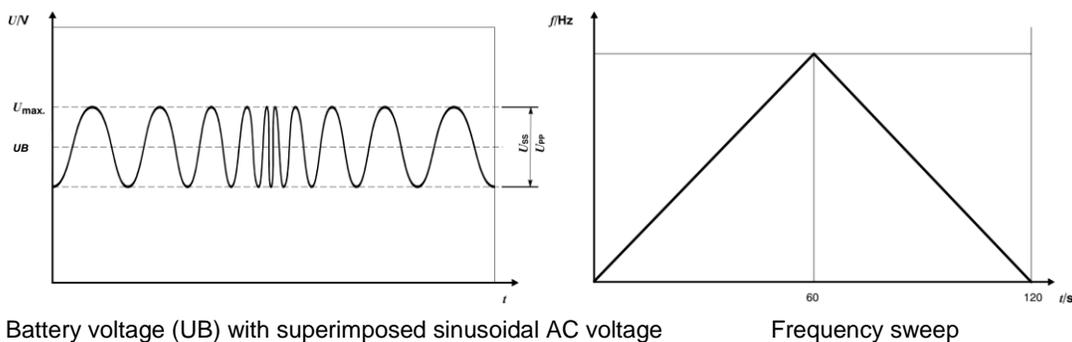
Frequency range: 50 Hz to 20 kHz, sine waveform, UB = 13.5V,
