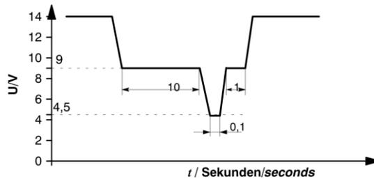
**Test conditions:**  $4.5 \text{ V} \leq UB \leq 9 \text{ V}$  for  $t \leq 100 \text{ ms}$ ; cycle time  $T \geq 20 \text{ seconds}$ ;
