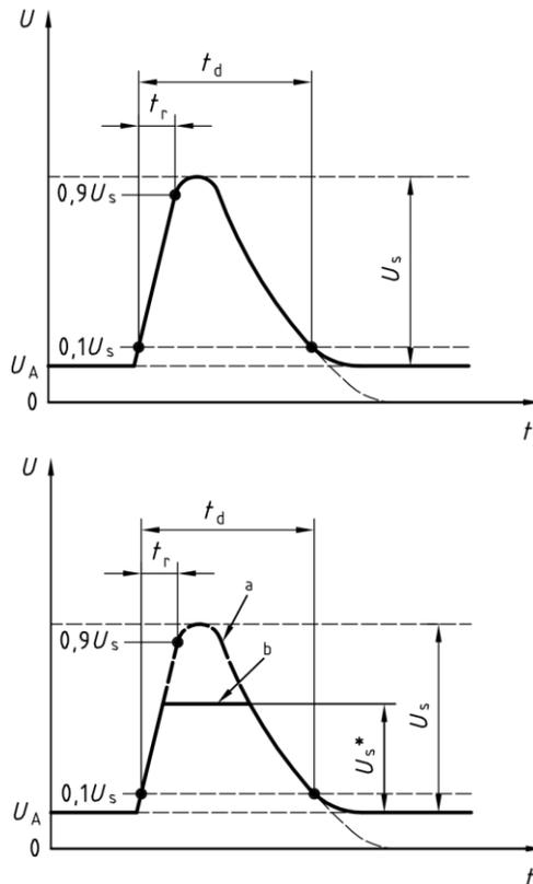
Parameters for test pulse 5a
