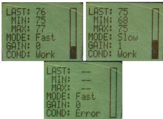
Examples during pulse measurement and when sensor is located outside human body.
