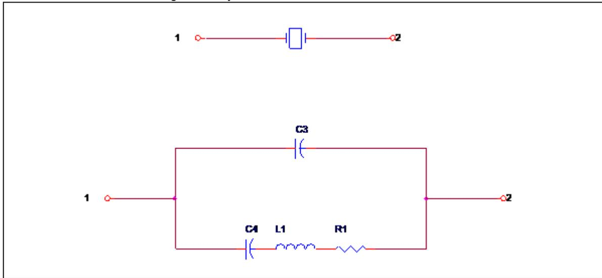
Many crystal manufacturers state a load capacitance in their part specifications. A load capacitance of 9 pF for a 26 MHz crystal means that the crystal is cut so that it will oscillate at 26 MHz, providing a 9 pF total shunt capacitance.
