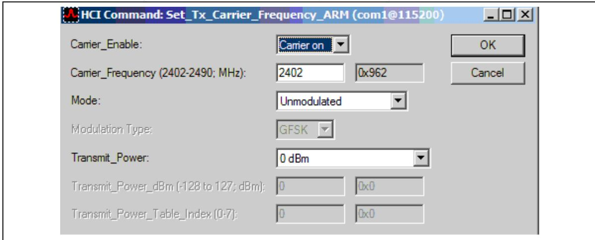
4. Measure the frequency of the carrier on the spectrum analyzer using a peak marker. If the measured frequency is below the expected value, decrease the values of either  $C_1$  or  $C_2$  or both. If the measured frequency is over the expected value, increase the values of either  $C_1$  or  $C_2$  or both.
