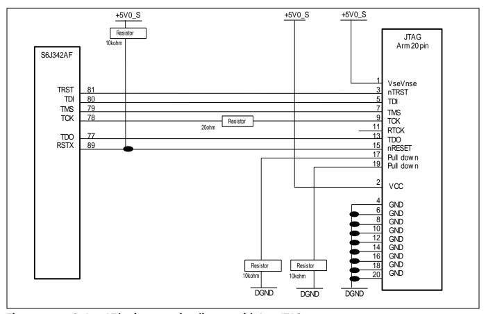
Figure 2 S6J342AF basic connection diagram with Arm JTAG 20
