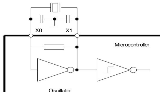
The following figure shows the general connection for an external main clock oscillator.
