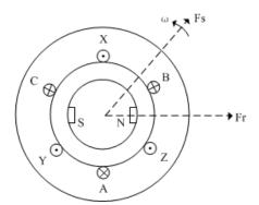
Figure 2. Structure of a 3-phase PMSM
