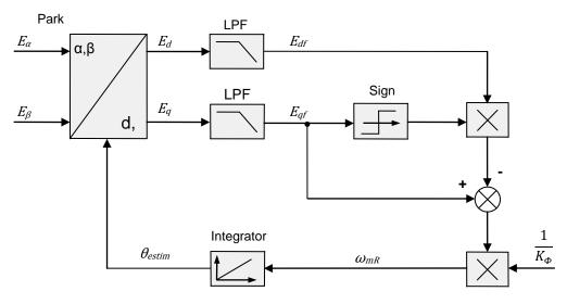
Starting from the closed loop shown in Figure 4-2, the estimated speed (wmR) of the rotor is integrated in order to obtain the estimated angle, as shown in Equation 4.4-1:
