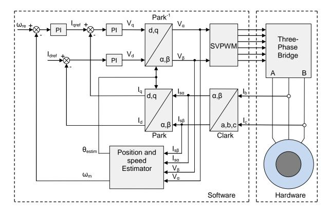
Figure 9. FOC Control Diagram
