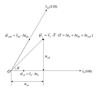
From the table of Eight Switching Statuses and Voltages, It is easy to know the basic vector amplitude is a constant  $(|\vec{v}_0| = |\vec{v}_{60}| = \frac{2}{3}V_{DC})$ .
