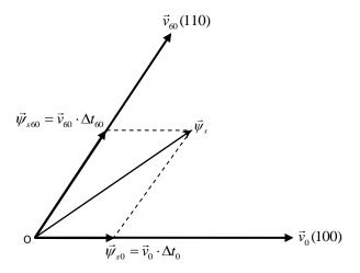
In above figure, it shows the synthesis vector in sector III. By the same way, the synthesis magnetic  $\vec{\psi}_s$  of any direction in every sector can be composed of the adjacent 2 basic vectors and the zero vectors.
