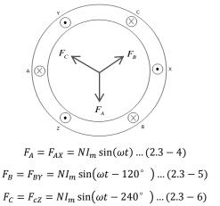
By observing the synthesis magnetic F in different timing modes, which is combined by  $F_A$ ,  $F_B$ , and  $F_C$ , it is easy to understand the rotating principle of stator magnetic field.
