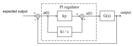
PI regulator causes a fluctuating output, fluctuating amplitude is decreasing. After some regulating periods, the output follows the expected output with a very small fluctuation around the expected output value.
