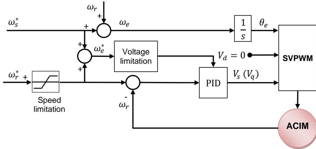
Figure 9 shows an alternative constant slip control scheme. Because current sampling is removed, a less expensive control is realized. Torque equation (2-9) suggests that when the slip speed is constant, the electrical torque is uniquely decided by V/f ratio. Thus the regulation target of a speed regulator could be V/f ratio or voltage, depending on the case of individual application.
