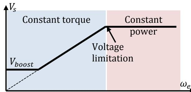
Figure 5 shows the stator voltage as function of synchronous speed in constant V/f control scheme. A boost voltage is added in low speed region when take reckon of voltage drop on resistance term. Depending on the specific system, the boost voltage could be designed differently to meet system requirement.
