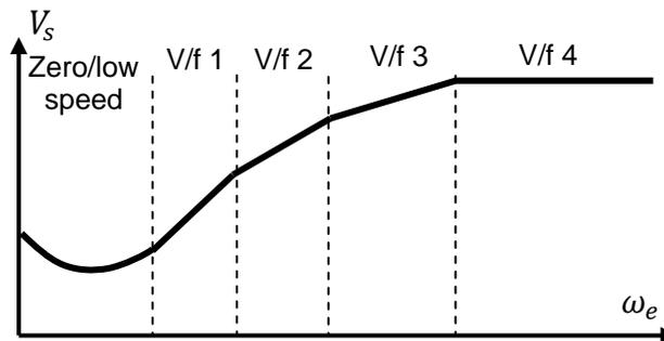
Other than single constant V/f curve, a varying V/f curve is preferred considering torque-speed characteristic.
