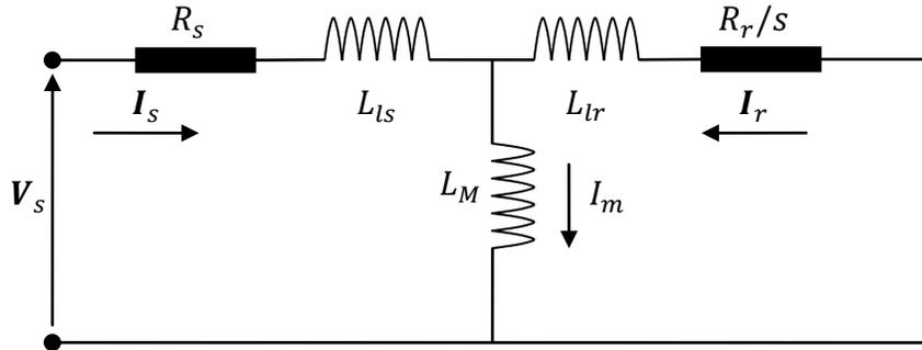
According to equation (2-1) ~ (2-4), stator voltage and current are related as
