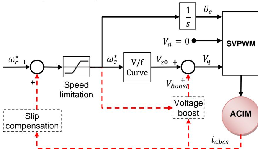
Figure 7. Speed Dependent Five-segment V/f Curve
