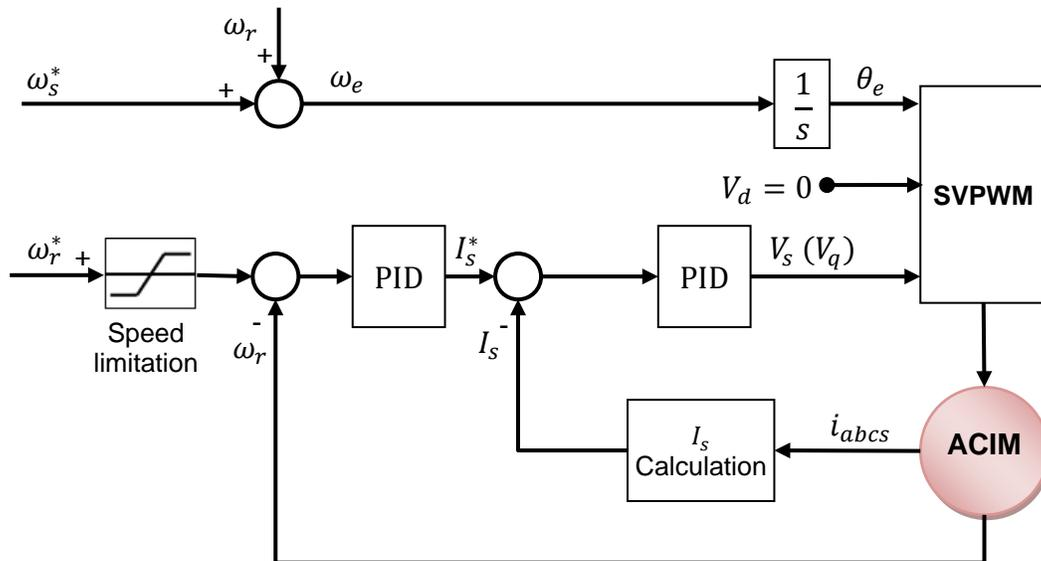
Figure 9. Constant Slip Control without Current Feedback
