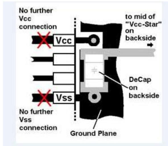
Figure 5 shows the recommended placement and routing if mounting on both sides is not possible.
