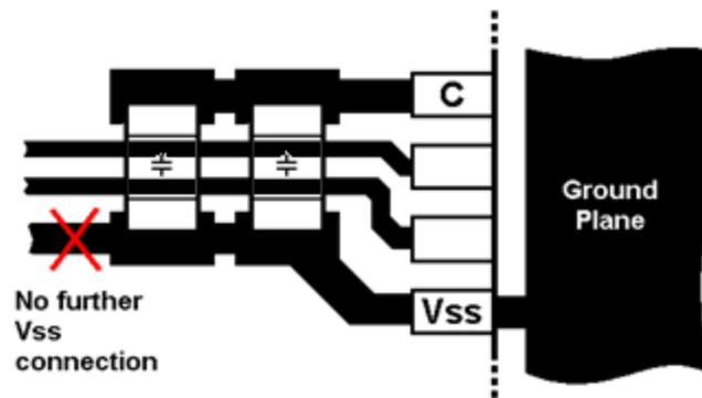
Figure 13 shows the recommended routing and placement for double sided metal layer. Note that despite the capacitor being placed on the opposite side from the MCU, this solution is preferred as the via to the ground plane and the via connecting to the C pin minimize inductance over other solutions.
