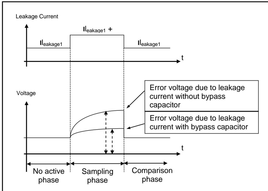
To show the effect of the bypass capacitor on reducing the leakage current error, we take a sampling time of 5  $\mu\text{s}$  and a leakage current of 3  $\mu\text{A}$  as an example. If we want to keep the voltage drop due to the second leakage current smaller than 0.5 LSB, the minimum size of the bypass capacitor should be chosen as:
