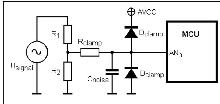
To protect the analog pins from suffering from an over-voltage, a “clamping resistor” is usually added to the input pins. The minimum value of the resistor can be chosen as
