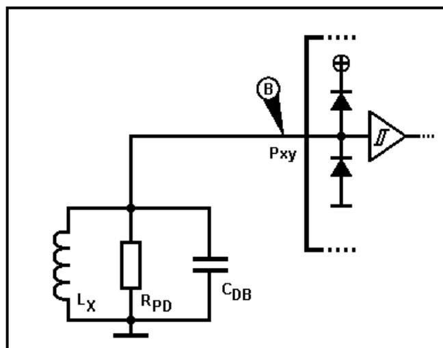
Because  $R_{PD}$  is often chosen high ( $> 50 \text{ k}\Omega$ ), its damping effect is weak.
