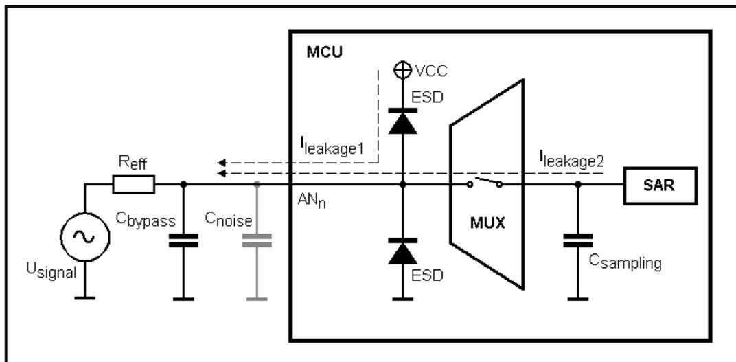
Figure 10. Error Voltage in the Sampling Phase
