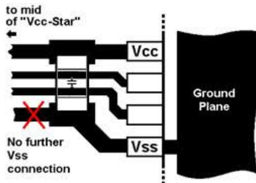
Figure 4 shows the recommended routing and placement for double-sided metal layers. Note that despite the capacitor being placed on the opposite side from the MCU, this solution is preferred over other solutions as the via to the ground plane and the via connecting to the  $V_{CC}$  pin minimize inductance.
