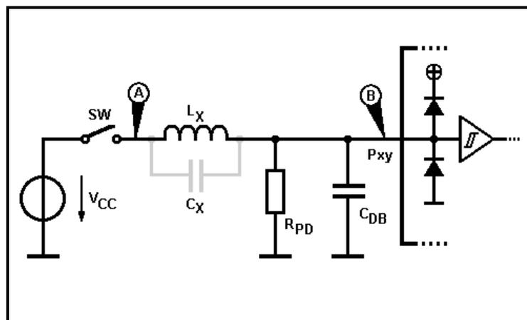
By closing the switch SW at time  $t_0$ , the voltage can be measured at point (A) in the above circuit as shown in Figure 19.
