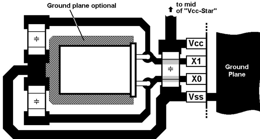
Figure 15 shows the quartz recommended placement and signal routing for a double sided metal layer layout.
