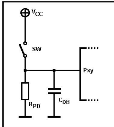
$R_{PD}$  is a pull-down resistor and  $C_{DB}$  is a debouncing capacitor. If the switch SW is open, a “0” is read from the port pin Pxy. If the switch is closed, the input changes to “1”.
