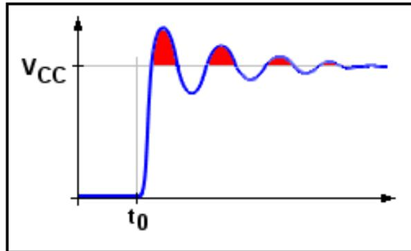
These overshoots may cause an internal latch-up on the port pin, because the internal clamping diode connected to  $V_{CC}$  becomes conductive. Opening the switch causes a similar result. In this case there are undershoots on the port pin.
