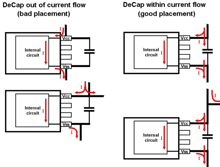
If possible, all decoupling capacitors should be placed on the same mounting side as the MCU. Cypress recommends 10 nF (~100 MHz resonance) to 100 nF (~10 MHz resonance) depending on the application.
