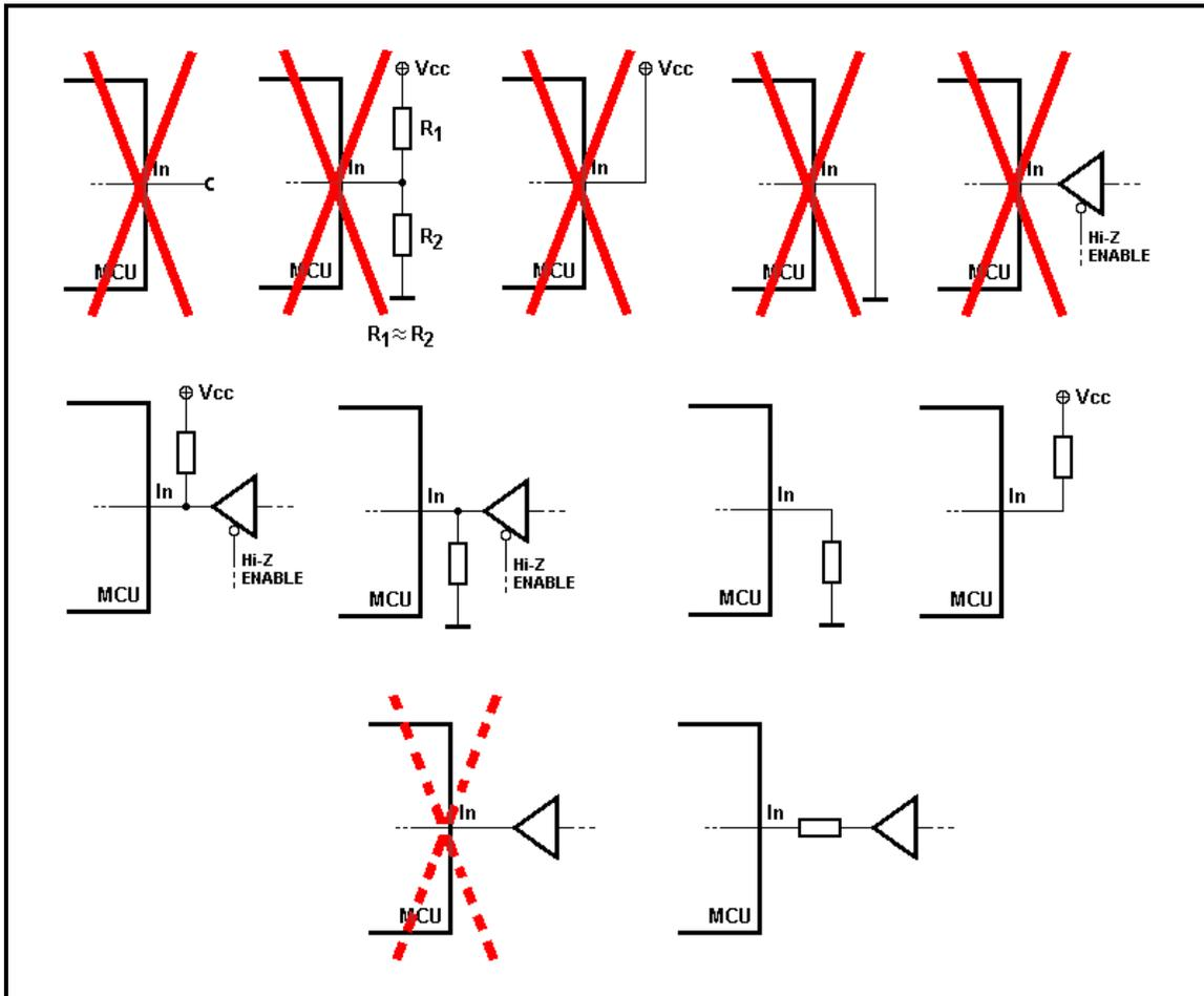
Be careful connecting input pins to other devices that can go into High-Z states. Always use internal pull-up or external pull-up or pull-down resistors in this situation.
