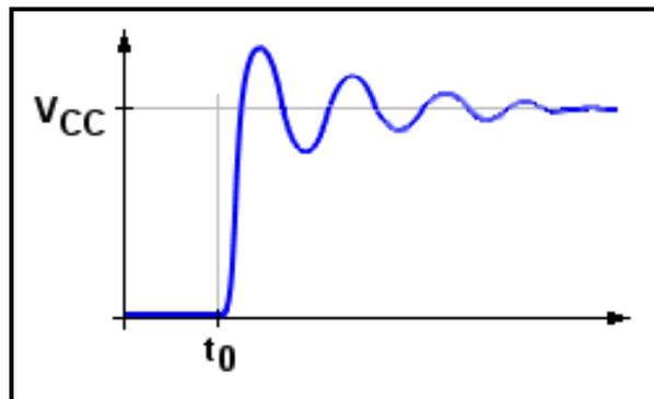
By closing the switch SW, (as in Figure 21) the circuit becomes a parallel oscillator with the wire-inductivity  $L_x$ , the debouncing capacity  $C_x$ , and the damping  $R_{PD}$  of the pull-down resistor, assuming the power supply to be ideal (no internal resistance).
