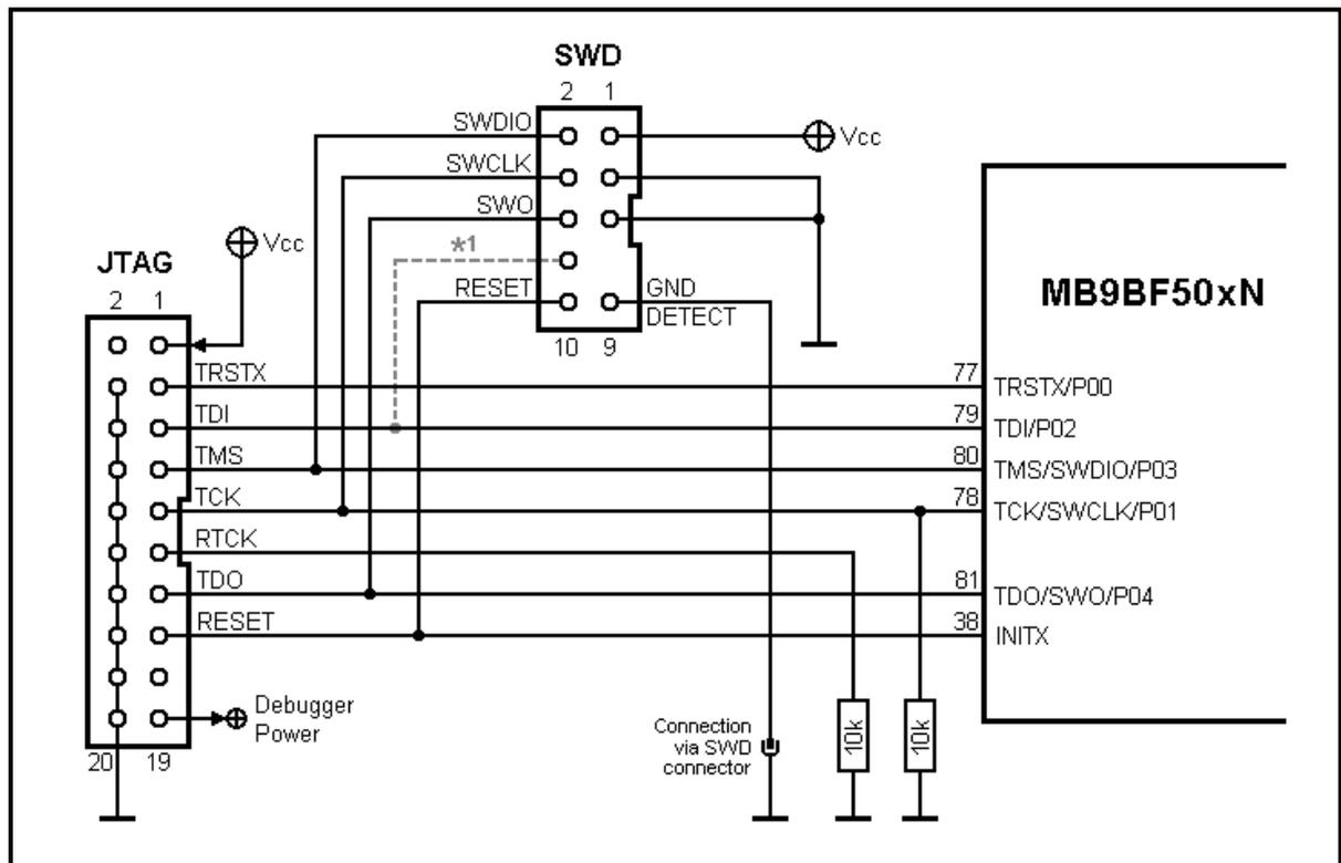
\*1 Only needed if SWD connector should also provide JTAG lines
