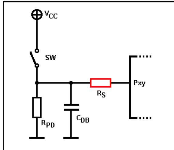
The series resistor  $R_S$  reduces the amplitude of the oscillation and decreases the voltage offset at first. The resistor must not be chosen too high, so that the port pin input voltage  $V_P$  is within the positive CMOS level. See [Figure 25](#).
