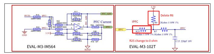
Figure 15 The PFC current feedback circuit for EVAL-M3-102T evaluation board
