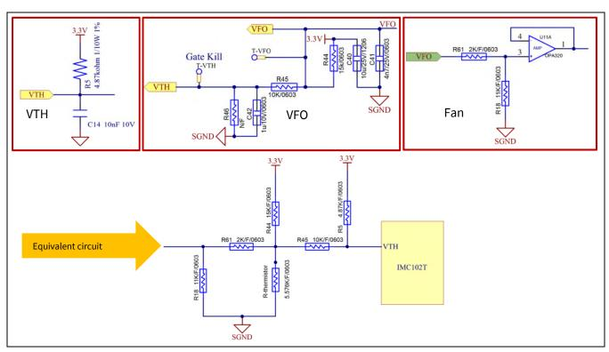
Figure 27 Overtemperature protection circuit schematic for EVAL-M3-IM564 and EVAL-M3-102T
