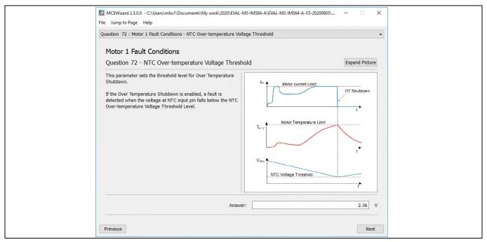
Figure 28 External temperature sense input configuration in MCEWizard
