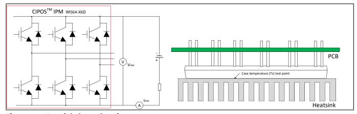
Figure 29 Heatsink thermal testing set-up
