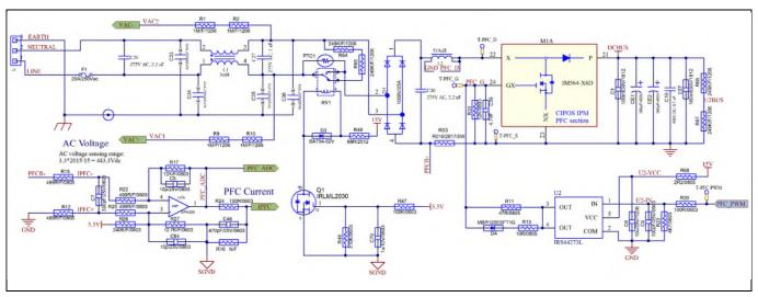
Figure 33 PFC section schematics for EVAL-M3- IM564
