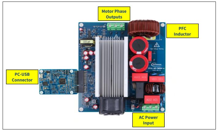
Figure 4 System connection example using EVAL-M3-IM564
