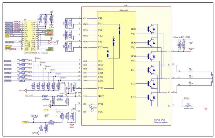
Figure 34 Inverter section schematics for EVAL-M3- IM564
