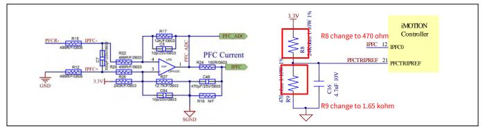
Figure 16 PFC OCP1 on the EVAL-M3-IM564 evaluation board
