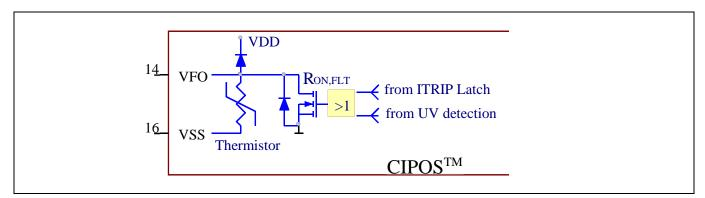
Figure 26 Internal circuit at pin VFO for CIPOS™ IPM IM564-X6D/IM564-X6DS
