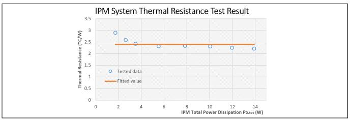
Figure 30 Heatsink thermal testing result
