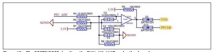
Figure 17 The PFCTRIPREF circuit on the EVAL-M3-102T evaluation board
