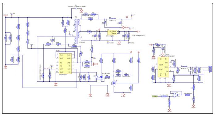
Figure 35 Auxiliary power supply section schematics for EVAL-M3- IM564
