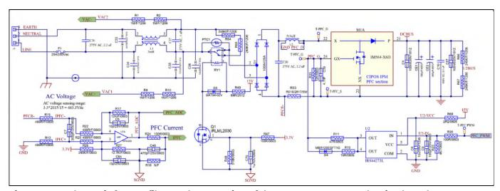
Figure 10 Schematic for EMI filter and PFC section of the EVAL-M3-IM564 evaluation board
