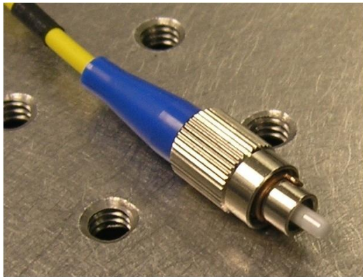
Figure 20. Ceramics FC connector
