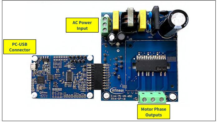
Figure 5 System connection example using EVAL-M1-101T and EVAL-M1-05-65D
