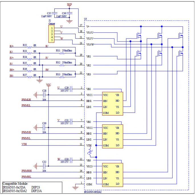
Schematic of the 3-phase inverter section using CIPOS<sup>™</sup> Micro on EVAL-M1-05-65D evaluation Figure 13 board
