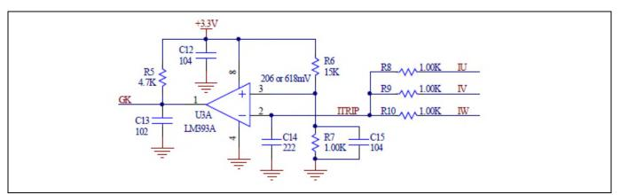
Over current protection circuit on the EVAL-M1-05-65D evaluation board Figure 15
