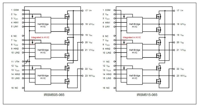
**CIPOS<sup>™</sup> Micro internal electrical schematic** Figure 2
