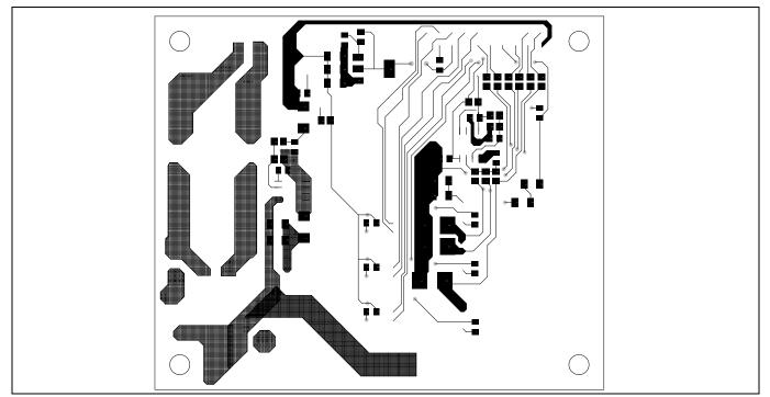
Figure 19 Bottom layer routing of the EVAL-M1-05-65D
