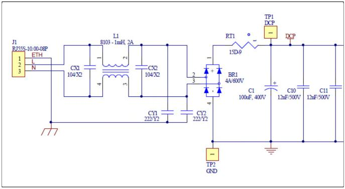
Schematic for EMI input filter and AC/DC section of the EVAL-M1-05-65D evaluation board Figure 12
