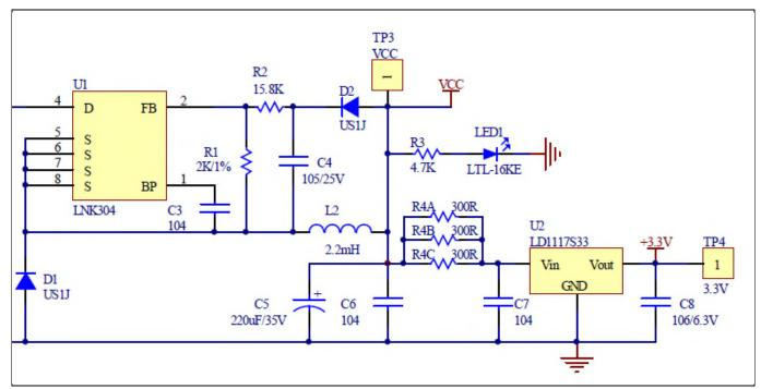
Power supply section of the EVAL-M1-05-65D evaluation board Figure 14
