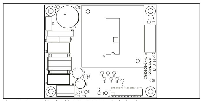
Figure 16 Top assembly print of the EVAL-M1-05-84D evaluation board
