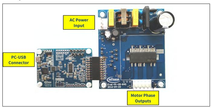
Figure 5 System connection example using EVAL-M1-101T and EVAL-M1-05-84D
