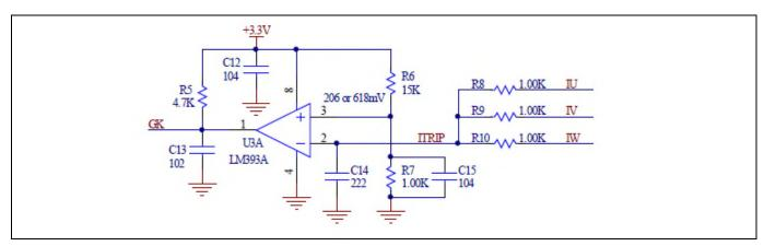
Figure 15 Over current protection circuit on the EVAL-M1-05-84D evaluation board
