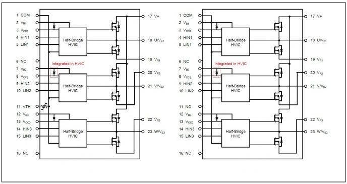
Figure 2 CIPOS™ Micro internal electrical schematic
