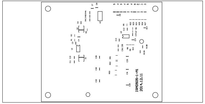
Figure 17 Bottom assembly print of the EVAL-M1-05-84D evaluation board
