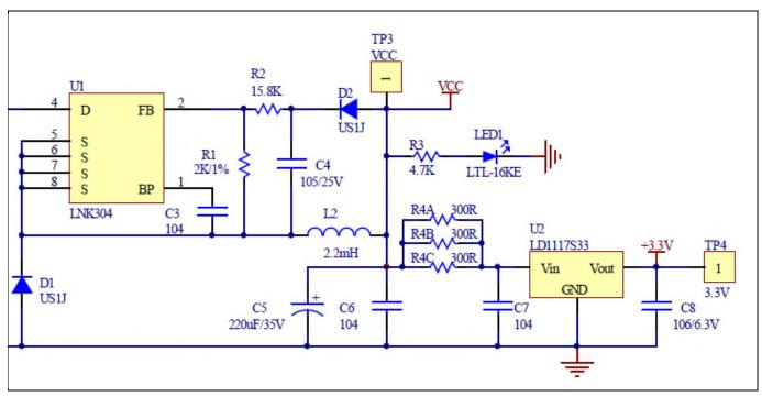
Figure 14 Power supply section of the EVAL-M1-05-84D evaluation board
