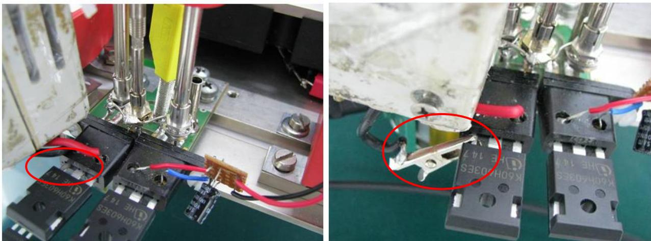
**Figure 1: On the left side the classical connection is illustrated. On the right hand side instead the connection with crocodile clip on the emitter pin is shown, causing lowering of the lead inductance value.**
