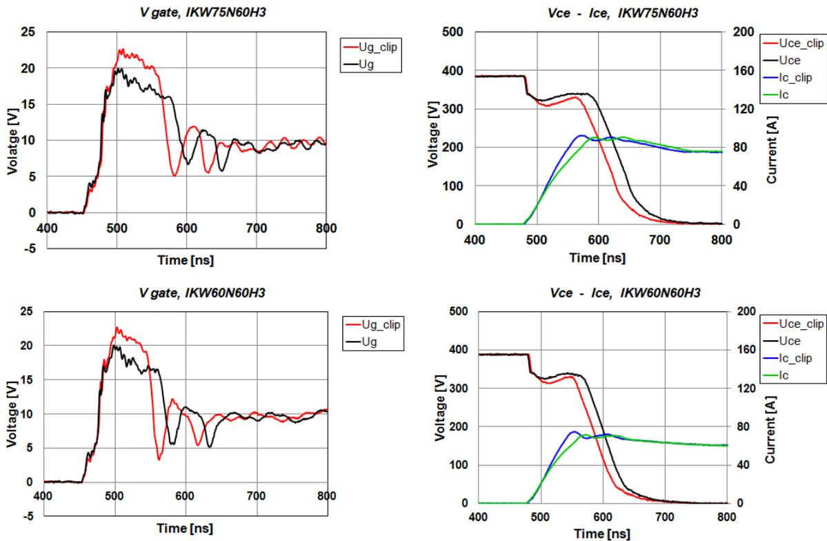
**Figure 2: IKW75N60H3 and IKW60N60H3 turn-on switching waveform comparison between simple plug-in and crocodile clip connection.**
