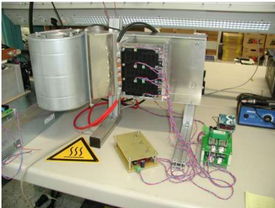
Figure 9: Test bench for IR-measurement done with an EconoPACK™ +
