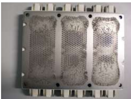
Figure 11: Optical appearance of a TIM-Layer after cycling. View to the base plate
