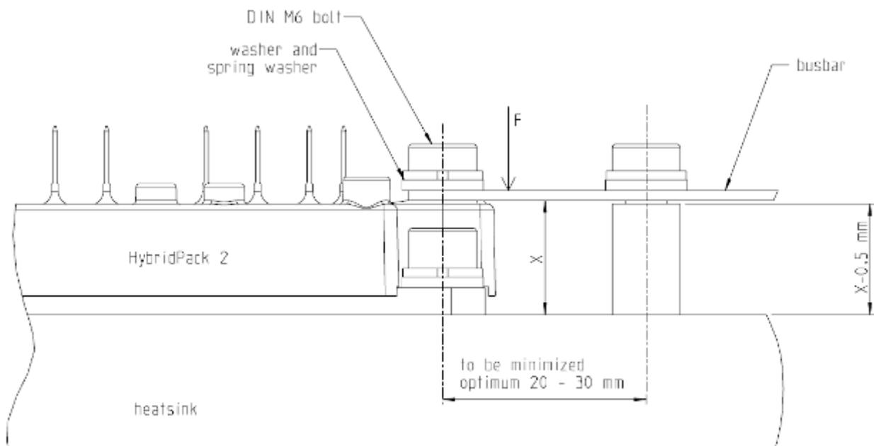
**Figure 11** Concept drawing of HybridPACK™ 2 assembly with ideal strain relief
