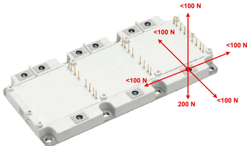
**Figure 10** Maximum permissible static pull and push forces at the power terminal of the HybridPACK™ 2.
