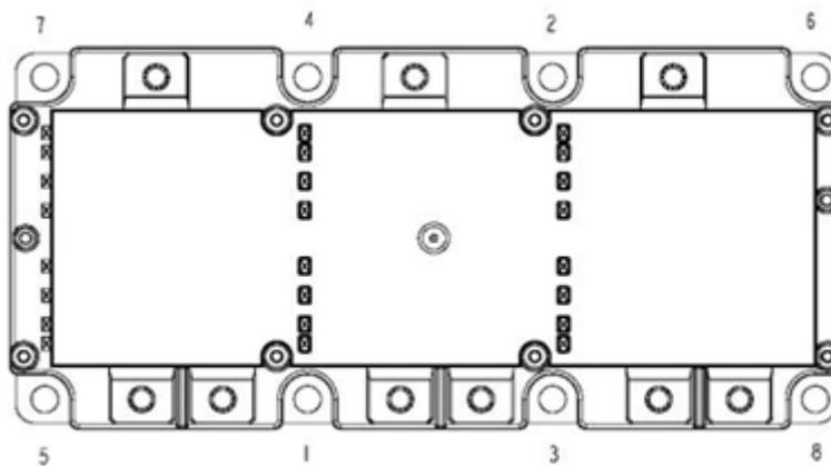
**Figure 9** Tightening sequence to mount the module.
