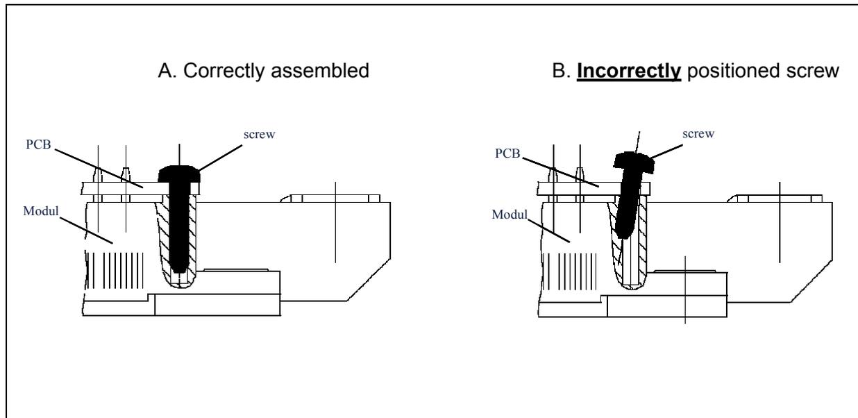
**Figure 3** (A) Correctly assembled screw into the mounting stand-off.
