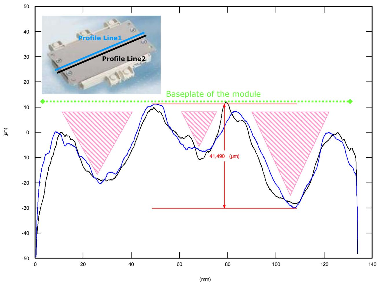
**Figure 6** Baseplate profile of a mounted HybridPACK™ 1 module (FS400R07A1E3).
