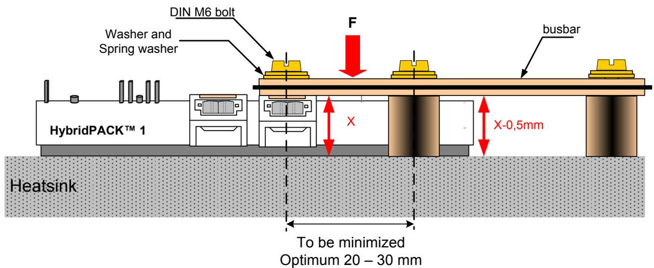
Figure 11 Concept drawing of HybridPACK™ 1 assembly with ideal strain relief
