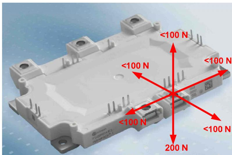
**Figure 10** Maximum permissible static pull and push forces at the power terminal of the HybridPACK™ 1.
