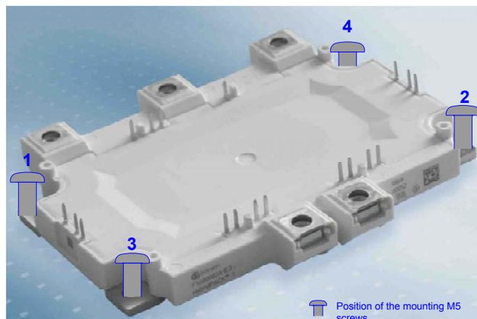
**Figure 9** Tightening sequence to mount the module.
