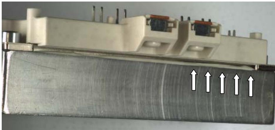
**Figure 4** Mounted HybridPACK™ 1 module with thermal compound squeezed out at the side
