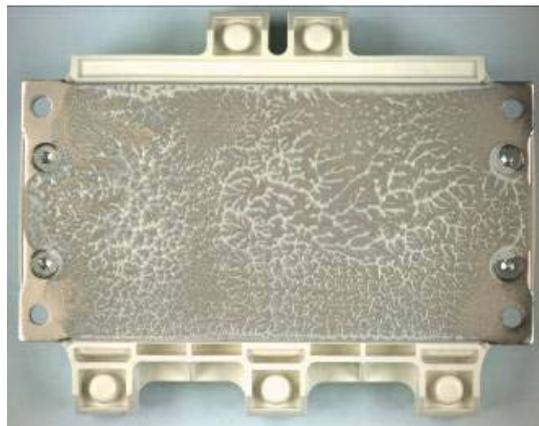
**Figure 5** Print image of a disassembled HybridPACK™ 1 with branch-like structure of the thermal compound
