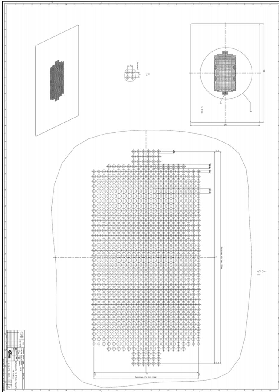
Figure 8 Screen print template for an HybridPACK™ 1 baseplate
