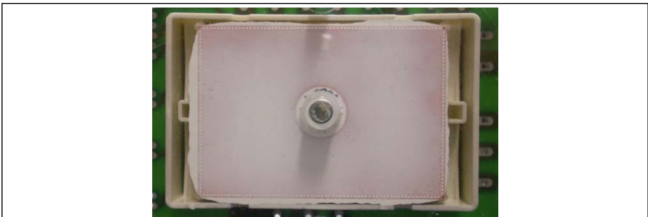
Figure 7 Mounted Smart1 Module with thermal paste visible at the module sides
