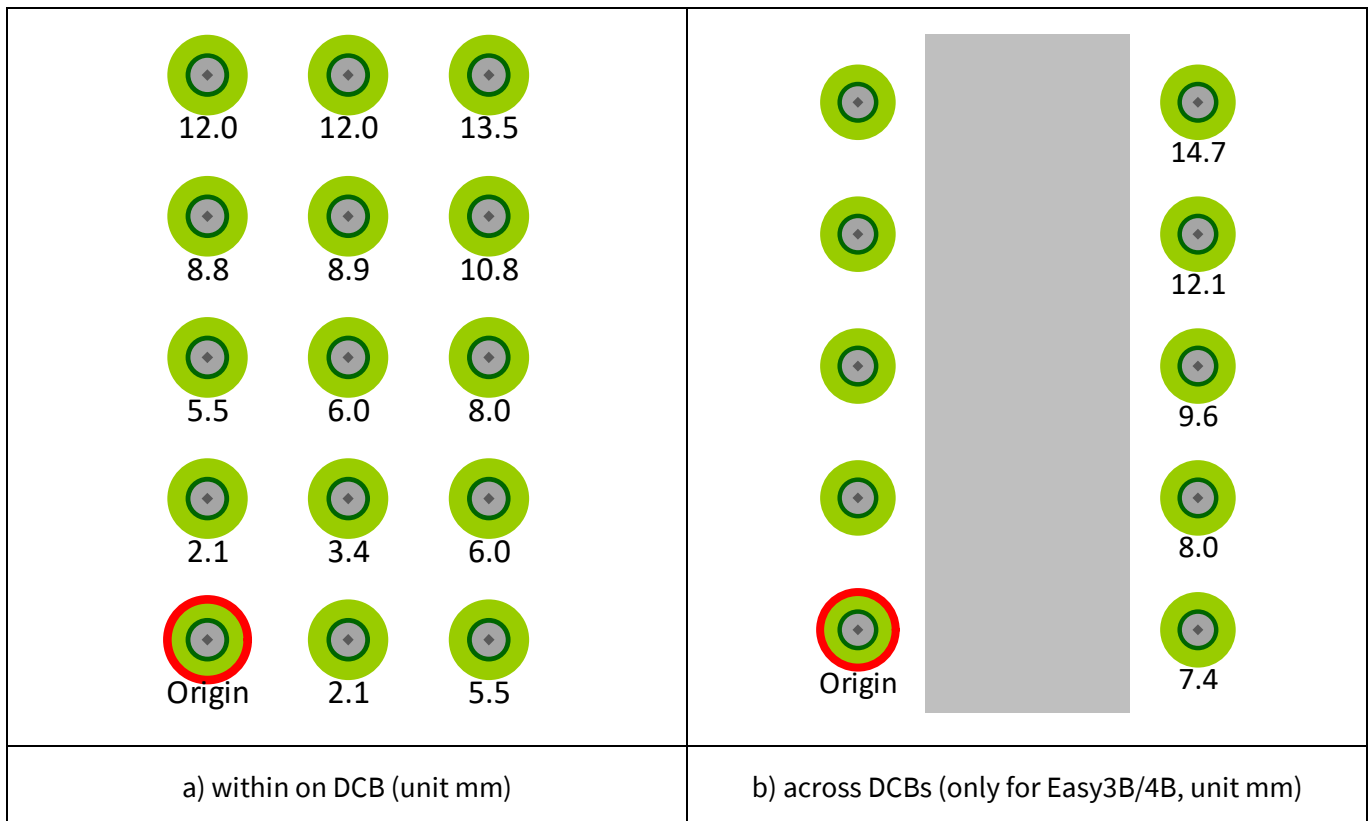
Figure 35 Pin-to-pin creepage distance for standard pins
