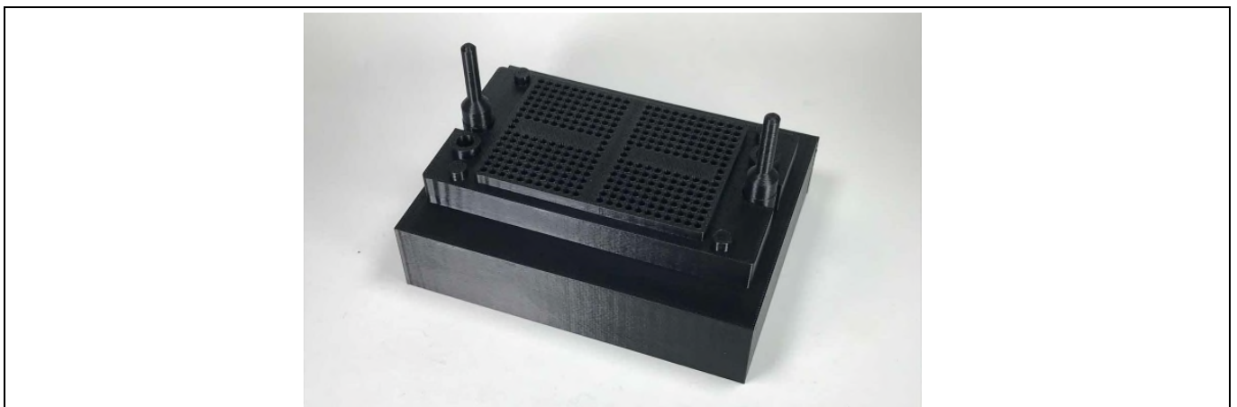
Figure 17 Press-fitting tools for Easy3B from HARTING Electronics GmbH
