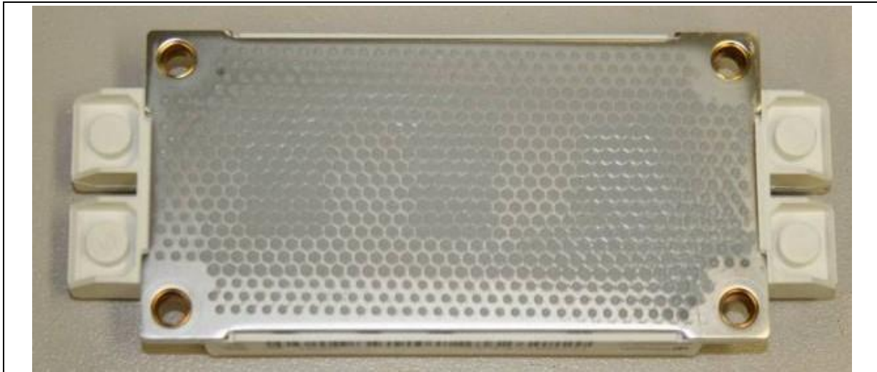
Figure 8 Base plate of an EconoDUAL™3 after applying TCP by screen printing
