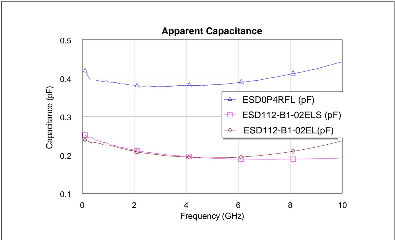
Figure 5 Apparent parallel capacitance of ESD0P4RFL and ESD112-B1
