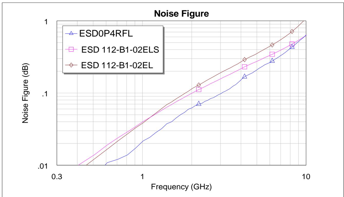
Figure 10 Noise figure of ESD0P4RFL and ESD112-B1
