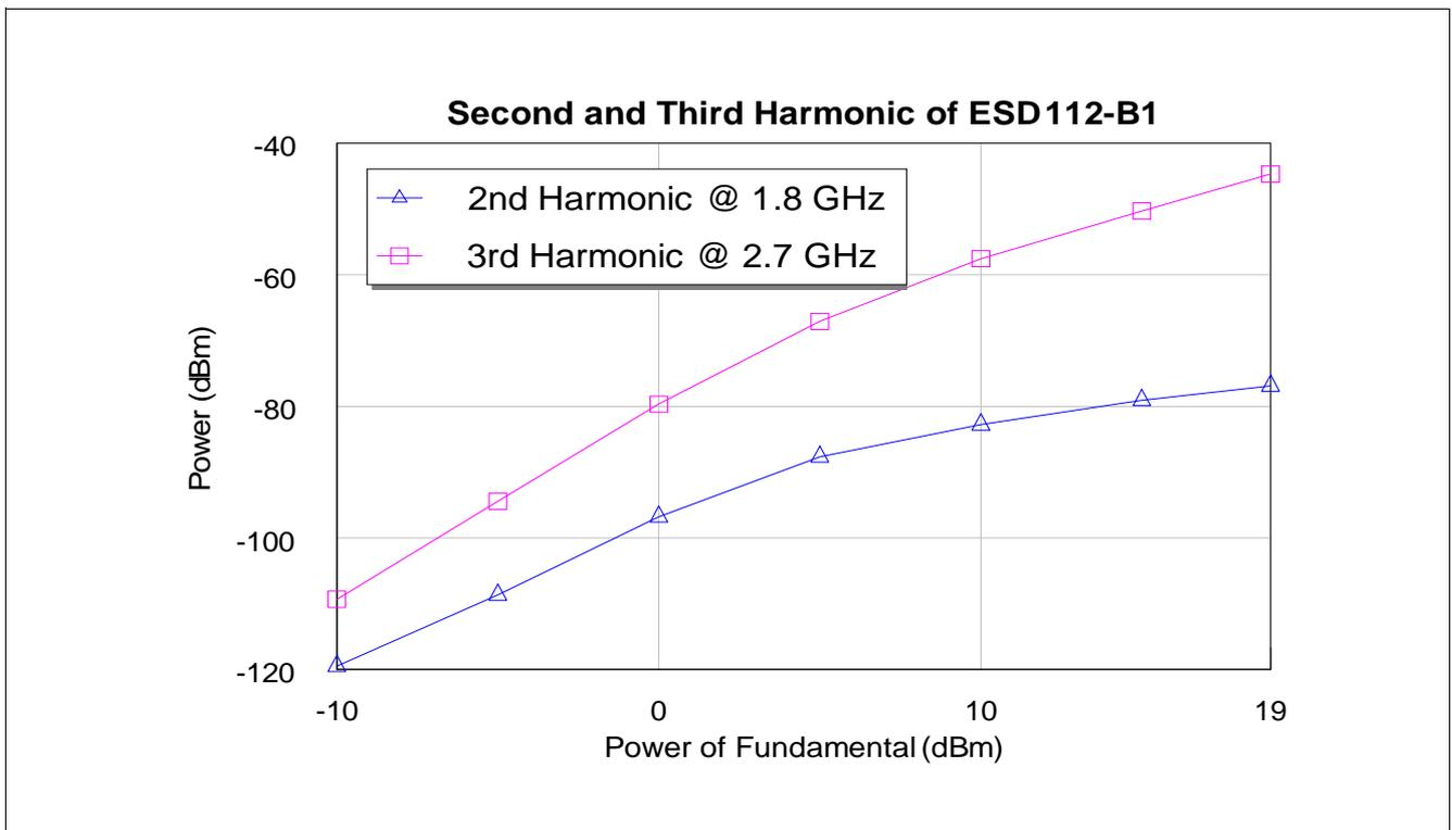
Figure 15 Harmonics generated by ESD112-B1 in steady-state from a fundamental tone at 900MHz in a 50Ω environment
