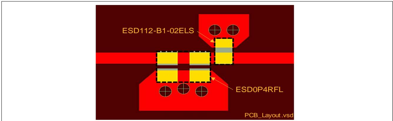
**Figure 22** PCB layout example for ESD112-B1-02ELS and ESD0P4RFL
