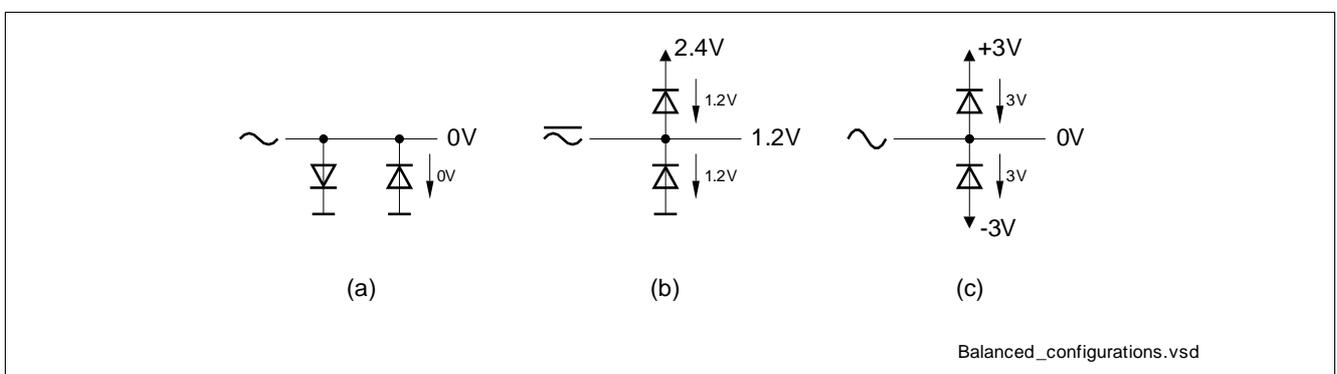
**Figure 13 Examples of balanced configurations of two diodes: (a) anti-parallel configuration, (b) rail-to-rail configuration with superimposed DC voltage on signal line and (c) rail-to-rail configuration with negative bias voltage**
