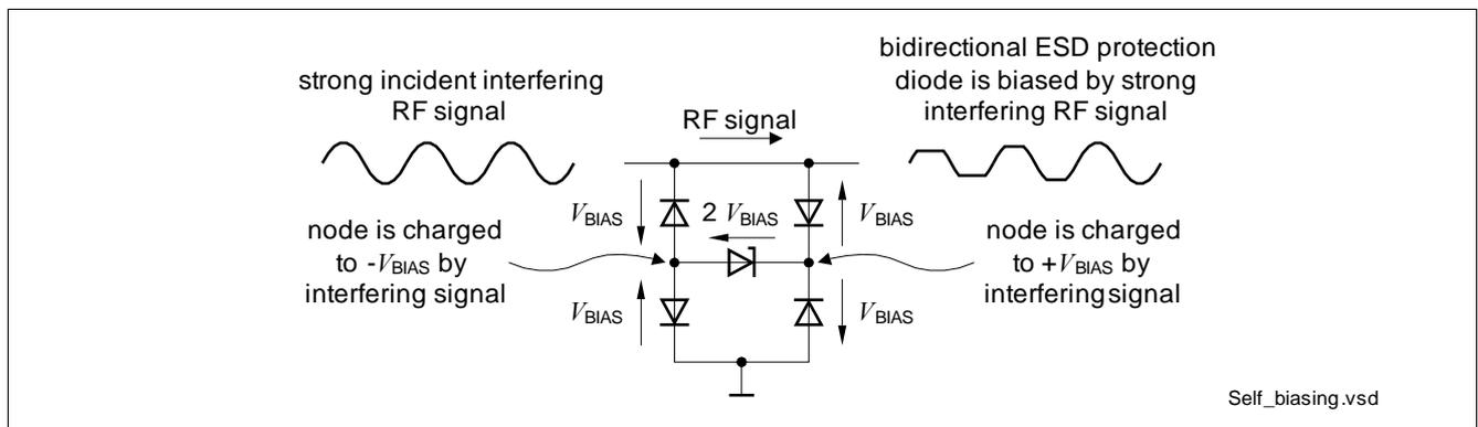
**Figure 16 Self-biasing of bidirectional ESD protection diode**
