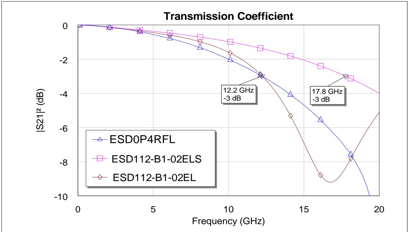
Figure 11 3dB bandwidth of ESD0P4RFL and ESD112-B1
