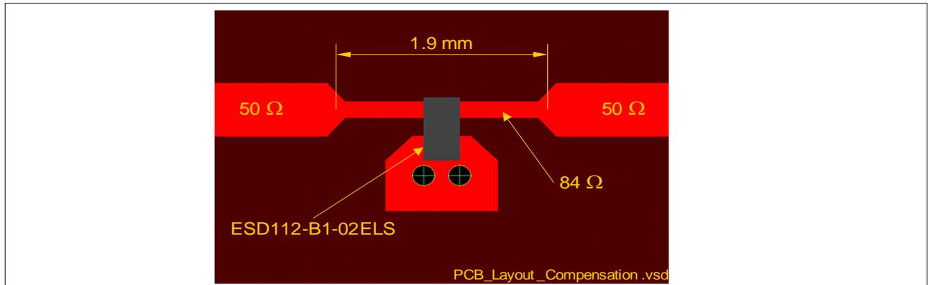
**Figure 27** Layout example on how the small capacitance of ESD112-B1-02ELS can be compensated
