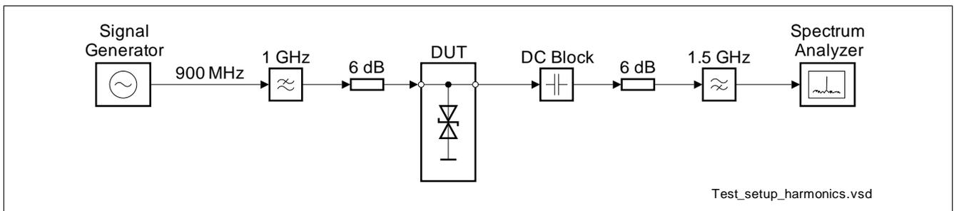
**Figure 12 Test setup for harmonics measurements**
