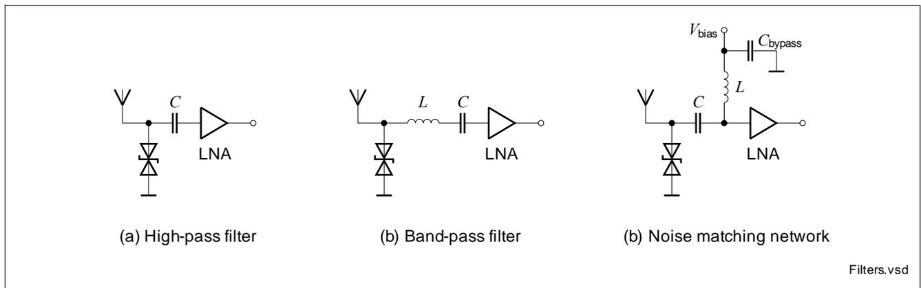
**Figure 23** Three different techniques for decoupling of ESD protection diode and LNA: (a) simple DC blocking capacitor as 1<sup>st</sup> order high-pass filter, (b) band-pass filter for applications operating around 100MHz or lower and (c) noise matching network as 2<sup>nd</sup> order high-pass filter
