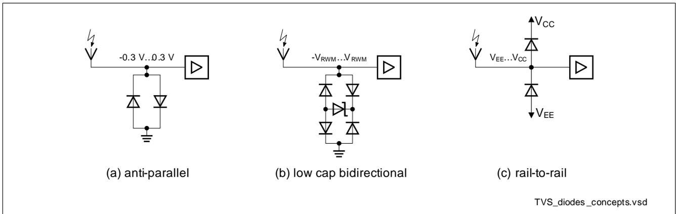
**Figure 3** Three different concepts for ESD protection diodes: (a) two low-cap diodes in anti-parallel configuration, (b) combination of four low-cap diodes and one Zener-like diode to a bidirectional configuration and (c) two low-cap diodes in rail-to-rail configuration
