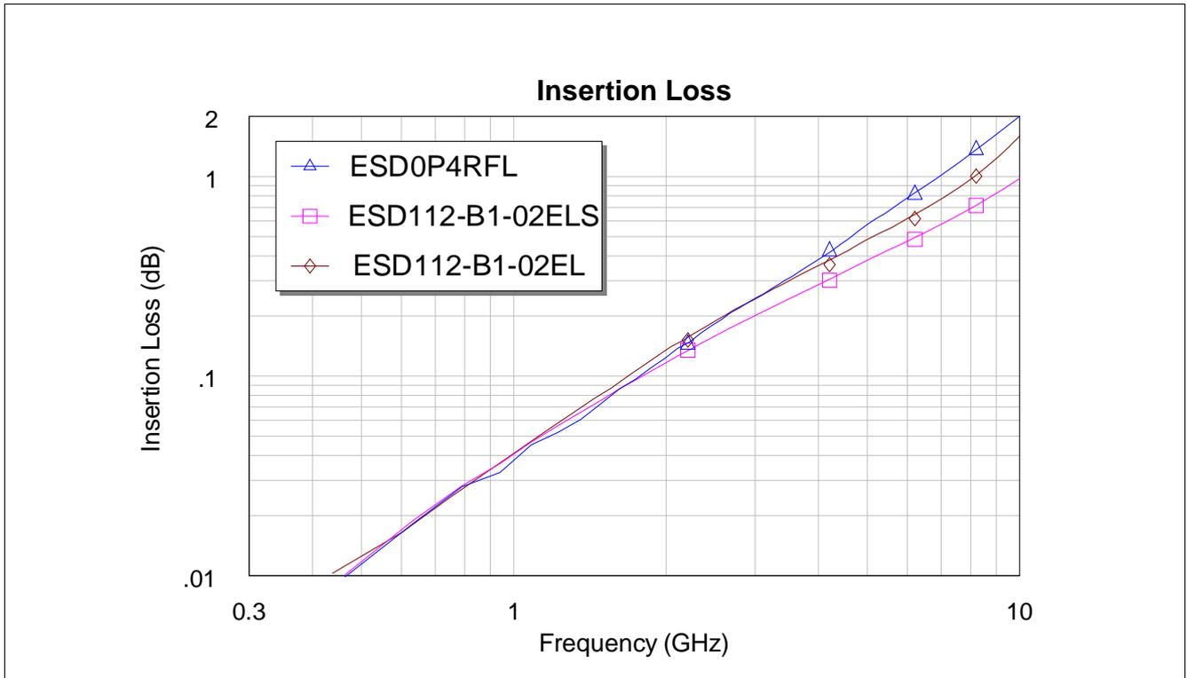
Figure 8 Insertion loss of ESD0P4RFL and ESD112-B1
