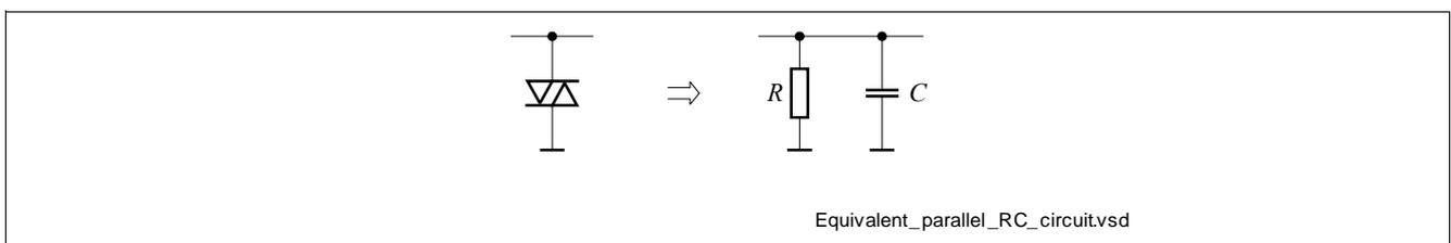
**Figure 4** Equivalent parallel RC circuit
