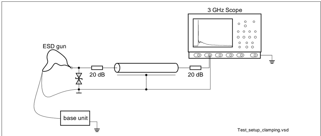
**Figure 17 Test setup for clamping voltage measurements**
