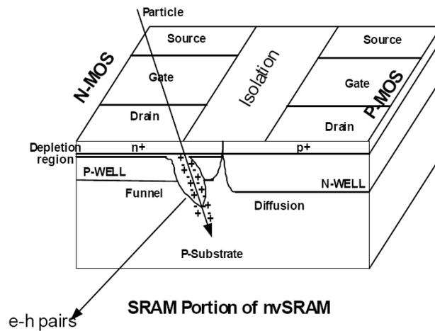
Figure 2. SRAM Cell in the nvSRAM
