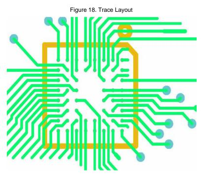
High-speed USB PCBs must be designed to meet USB electrical requirements. This is best achieved by using controlled impedance PCBs, properly laying out D+ and D–, and adequately decoupling the VCC and GND planes to keep them electrically quiet.
