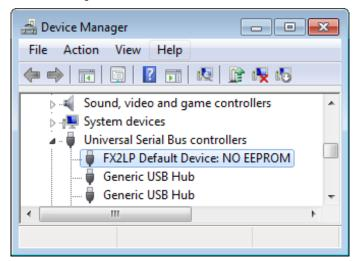
**Note:** You can also install the driver using an FX2LP development board (available here) with its EEPROM ENABLE slide switch set to the NO EEPROM position. This enables the default device with VID=0x04B4 and PID=0x8613.
