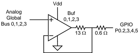
The 13Ω represents the dynamic output impedance of the buffer opamp. The closed gain drives the output voltage very close to the input, resulting in essentially zero output impedance until the lower output device (an N-channel FET) is driven all the way on. At this point it looks like 13 Ω. The 0.6-Ω resistor represents the resistance of the on-chip routing and the bond wire.
