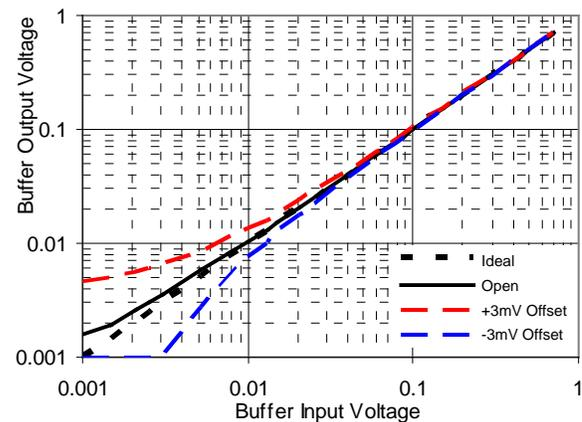
With no load, the buffer output drive limit is the offset voltage. If the load is to circuit ground ( $V_{SS}$ , not AGND), the output still follows the slope of Figure 1.
