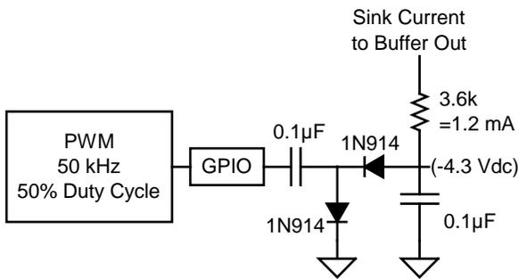
This circuit provides the sinking current near the rail. With the original configuration - a 9-bit DAC and a 1.0 mA pull up load - the buffer could not get down to the required voltage. Adding a 1.2 mA pull down current (3.6 kΩ to negative source), the output now swings all the way to  $V_{SS}$ , as shown in Figure 6, tracking the unloaded output all the way to the rail.
