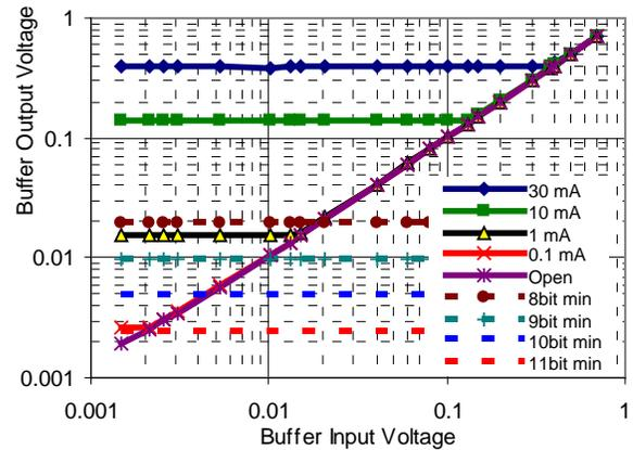
This shows that you can meet the required minimum output voltage level for a 9-bit converter only if the sinking current is less than 700 µA. This may not be enough drive current for a typical application. A typical example is a resistive load terminated to V<sub>DD</sub>/2 or a capacitive coupled load, which results in a maximum resistive load of 2.5 V/0.7 mA = 3.48 kΩ. An example circuit is DAC output for a synthesized signal driven to the zero code at the bottom of its range.
