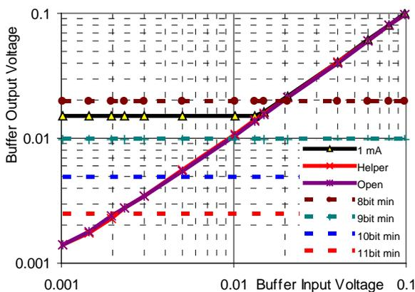
The pull-down resistor draws current all the time. When the basic Class-A output is at AGND (for example,  $V_{DD}/2$ ), there is  $2.5\text{ V} + 3.6\text{ V} = 6.1\text{ V}$  on the resistor for an average current addition of 1.7 mA when the pull down helper is set for 1.0 mA. The design must be able to accommodate this additional current draw. To reduce power, the PWM can be disabled when the DAC output is not required to drive to the rail.
