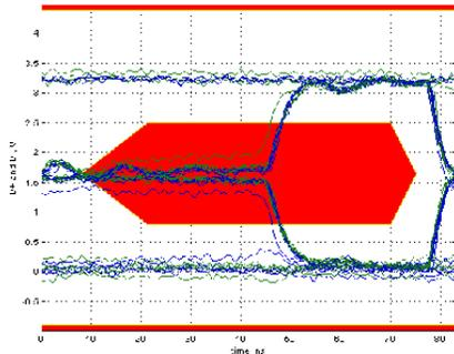
Another typical mistake when working with high-speed signals is connecting the differential probe backward. This causes the image that appears in Figure 3.
