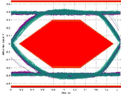
The signal is not only affected in the rise time but also with a slight increase in jitter. If the design were to add up to 8 pF, it would start to show signs of eye violations. When inductance is added to the traces, the signal has an overshoot and may round off both the top and bottom of the eye.
