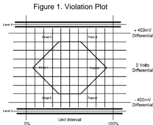
The signal must not pass through the violation area. If it does, at least one of the USB specification requirements has been violated. The limits of the violation area depend on the configuration of the device being tested. If the device has a “captive” cable, it has a different set of limits than a device that has a standard B connector. The USB-IF specification contains the plots for each of these tests. After the proper test limits have been selected for the
