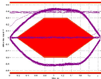
This happens because the scripts that synchronize to the data patterns make an assumption about the probe's polarity. They expect the signals in a specific sequence. When the signals are reversed by connecting the probe 180 degrees out, they measure the D+/D- differential pair as a D-/D+ differential pair. This causes the algorithm to plot the leading edge of the signal, which creates the lines through the center. Reversing the probe connection removes this problem.
