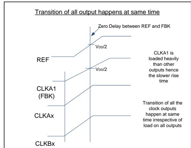
Hence, changing the load on an output changes its rise time and therefore how long it takes the output to reach the  $V_{DD}/2$  threshold. According to these properties, the outputs can be advanced by loading the feedback output heavier than the other outputs, or they can be delayed (lagged) by loading the feedback output lighter than the other outputs. This is explained in Figure 3.
