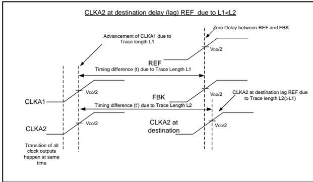
As with any buffer, individual clocks may be advanced by shortening that particular trace, or delayed by lengthening it. When lengthening traces, beware that a tight serpentine routing adds less delay than an equal length trace that does not bend back on itself. This is because the closely routed trace couples to itself, which helps to speed the propagation of the signal.
