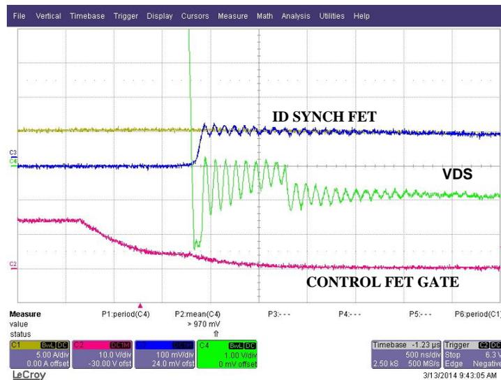
Figure 4: expanded time scale view of operating waveforms
