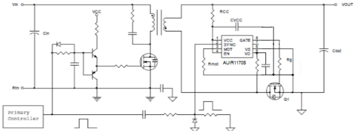
Figure 2 : Flyback converter with smart synch-rectification
