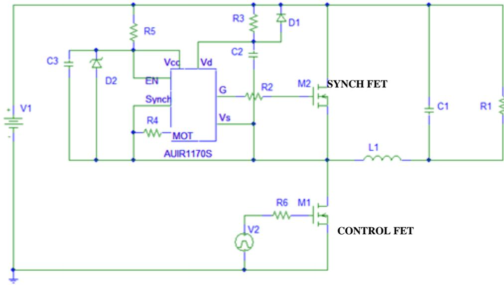
Figure 5: actual circuit used for hard switching tests
