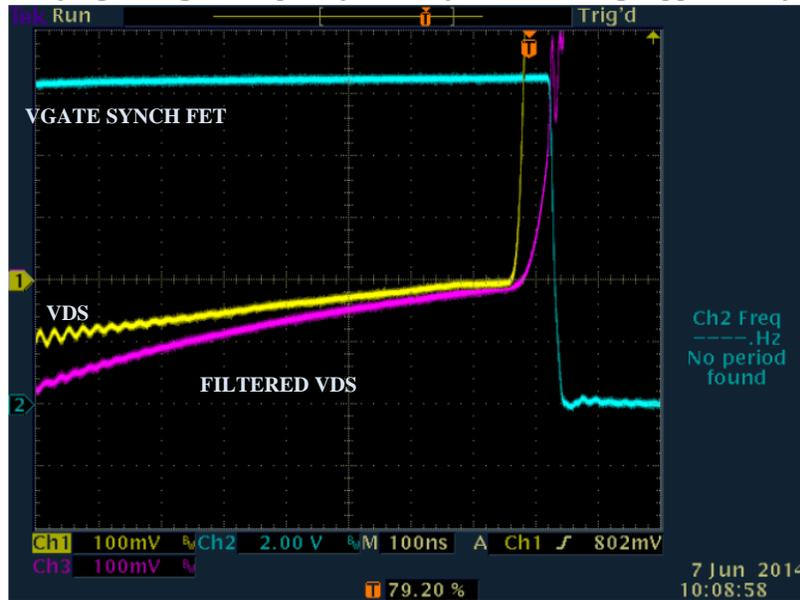
Figure 13: turn-off delay by 600kHz cutoff frequency filter.
