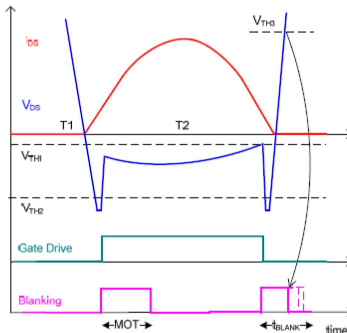
Figure 11: theoretical secondary waveforms for a resonant converter
