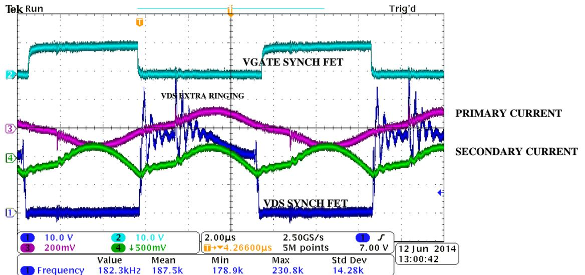
Figure 12: practical secondary waveforms in a LLC converter
