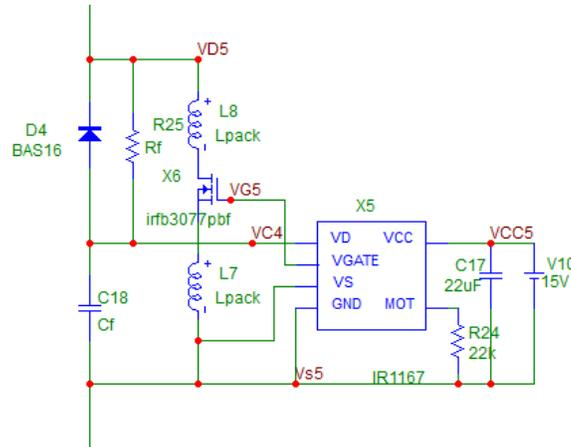
Figure 9 : Vds filtering for improved noise rejection
