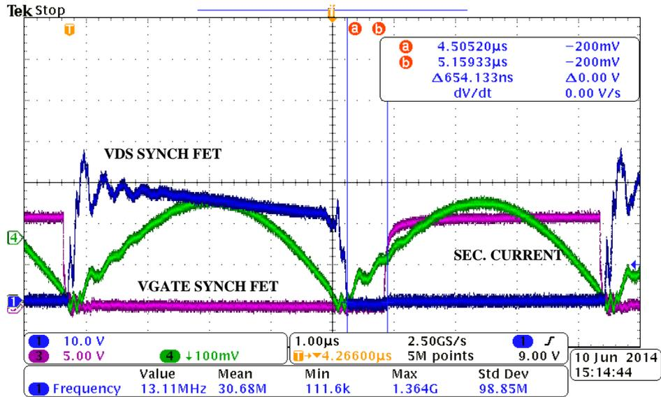
Figure 14: effect of Vds filter on turn-on delay.
