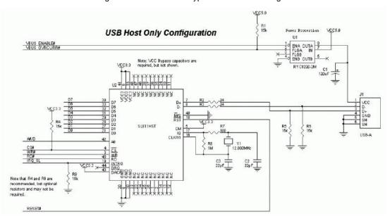
Figure 5. SL811HS in a Typical USB Host Configuration
