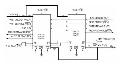
Figure 4. Width Expansion of Synchronous FIFOs (CY7C42x5)
