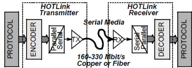
Figure 2. CY7B923 Transmitter Logic Diagram
