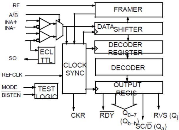
The SC/D (Special Character/Data) pin permits the transmission of command codes in addition to data characters. The codes are mapped to 10-bit transmission characters defined in the 8B/10B codes of the Fibre Channel standard. Commands can be sent as part of the transmission stream, to signal events such as Idle, Start-of-frame (SOF), End-of-frame (EOF), and so on.
