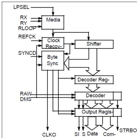
Figure 7. Am79168 and Am79169 Configurations
