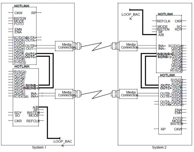
Figure 8. Example HOTLink Loop-Back System Connection
