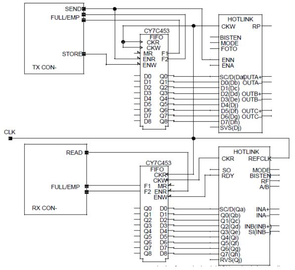
Figure 12. Clocked FIFO Interface (Note 2)
