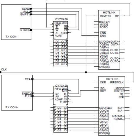
Figure 11. Asynchronous FIFO Interface<sup>(Note 1)</sup>
