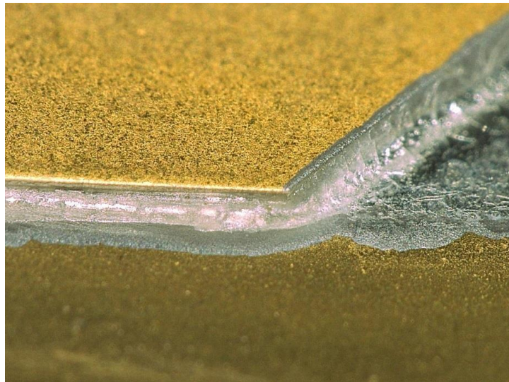
Figure 9 Non-wetting of the lead side walls is not a reject criterion
