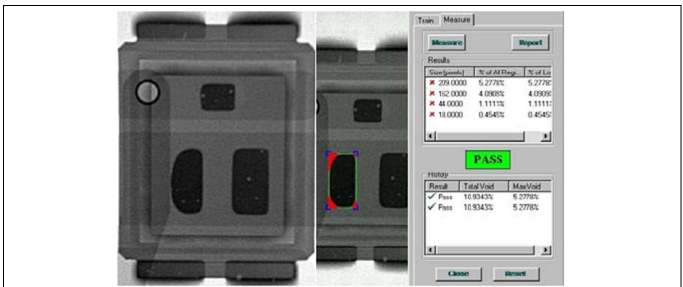
Figure 18 Poorly formed source joint - 11% missing
