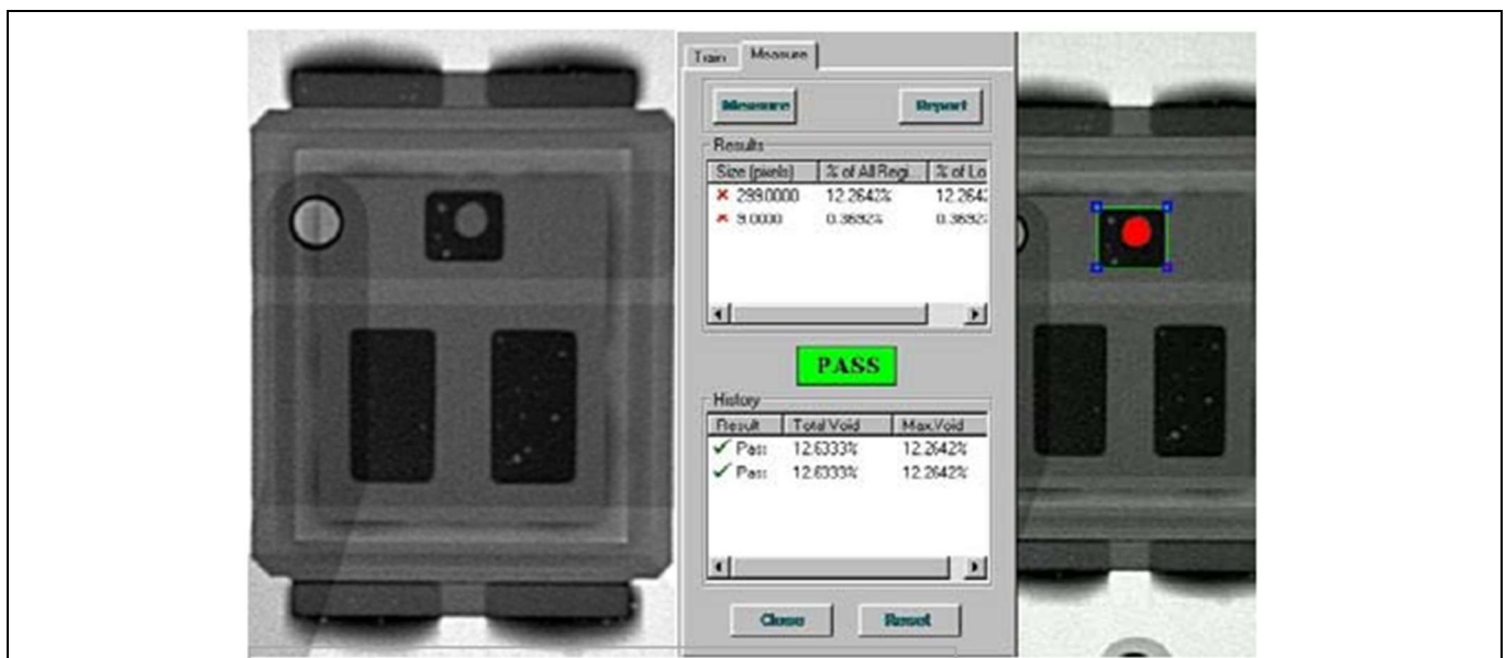
Figure 12 Voids on the gate contact
