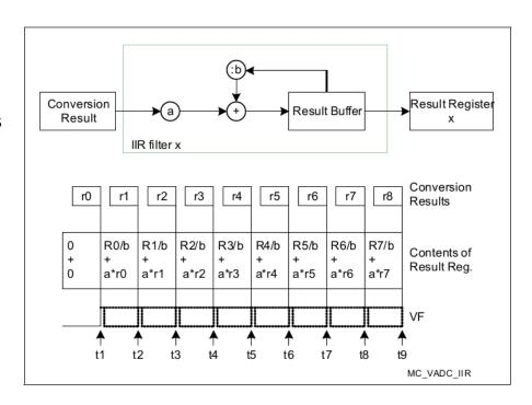
**Note:** In this example, a delay before starting to read the conversion results is needed. This ensures that incorrect values are not read due to the filters not being yet at full speed.
