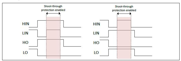
Figure 14 Illustration of shoot-through protection circuitry
