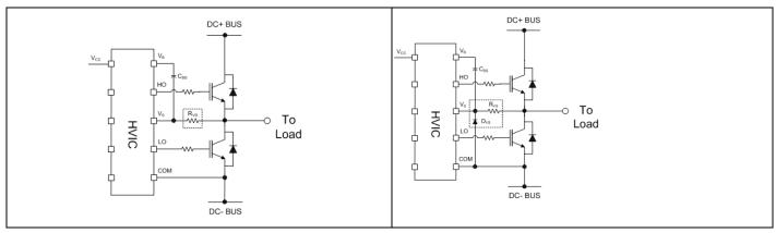
Figure 26 Resistor between the VS pin and the switch node
