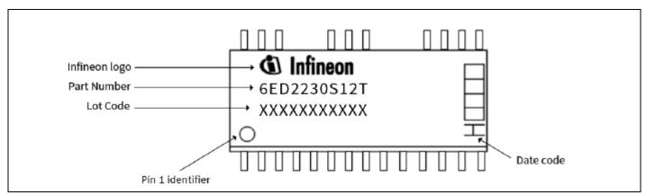
Figure 30 Marking information PG-DSO-24 (DSO-28 with 4 pins removed) [Marking Diagram to be updated]
