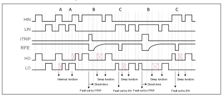
Figure 7 Input/output timing diagram
