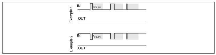
Figure 19 Noise rejecting input filters
