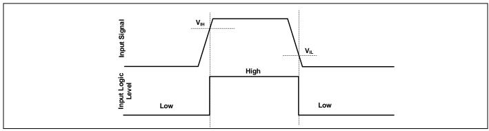
Figure 12 HIN & LIN input thresholds
