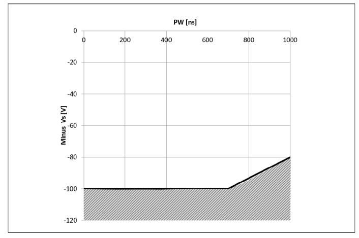
Figure 24 Negative Vs transient SOA for 6ED2230S12T @ VBS=15V
