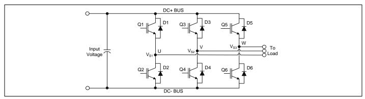
Figure 21 Three phase inverter
