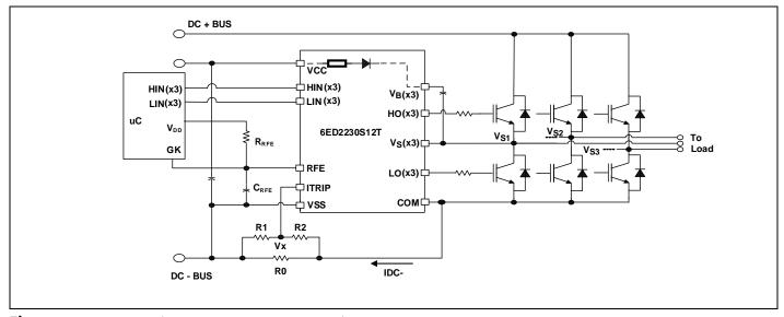
Figure 16 Programming the over-current protection
