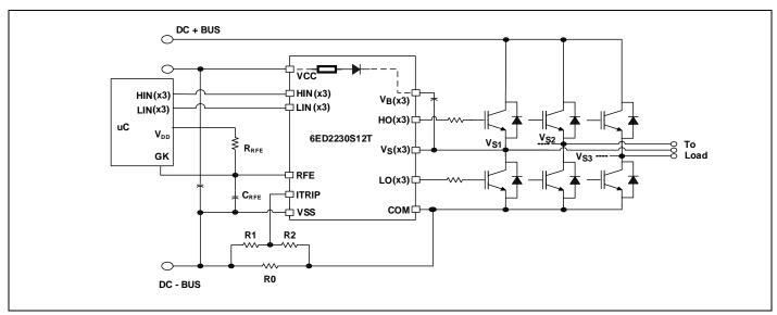
Figure 15 Programming the fault clear timer
