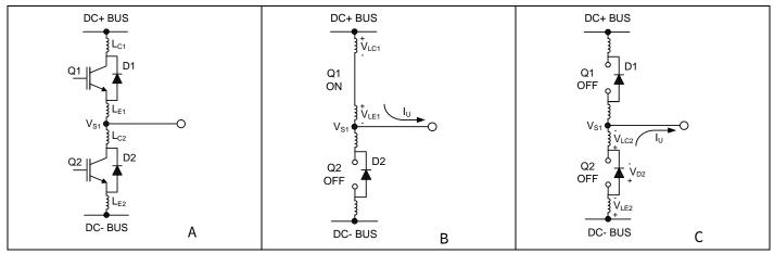
Figure 23 Figure A shows the Parasitic Elements. Figure B shows the generation of  $V_s$  positive. Figure C shows the generation of  $V_s$  negative
