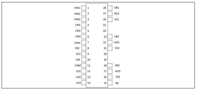
Figure 3 6ED2230S12T pin assignments (top view)
