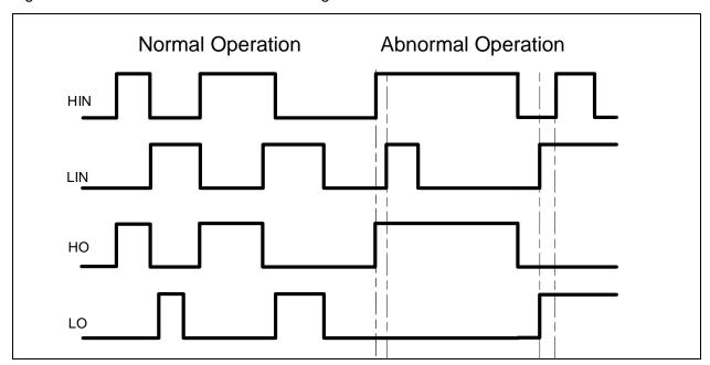
Figure 12 Illustration of shoot-through protection circuitry
