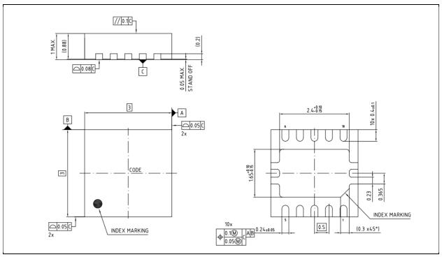
Figure 21 Target Package Dimensions: PG-VSON-10-5 (2ED2744S01G)
