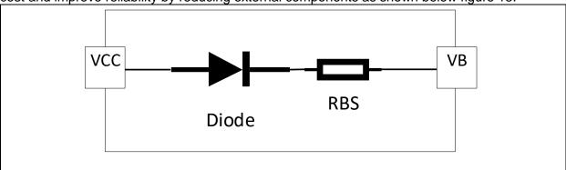
Figure 13 2ED2744S01G with integrated components
