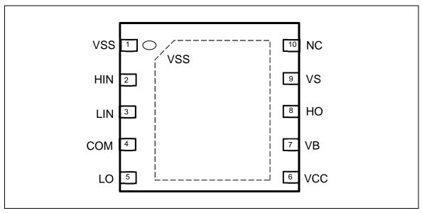
Figure 3 2ED2744S01G pin assignments (top view)
