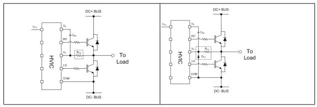
Figure 19 Resistor between the VS pin and Figure 20 Clamping diode between COM the switch node and  $V_S$
