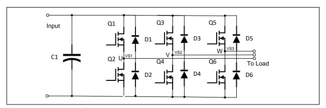
Figure 15 Half bridge inverter
