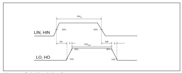
Figure 6 Switching timing diagram
