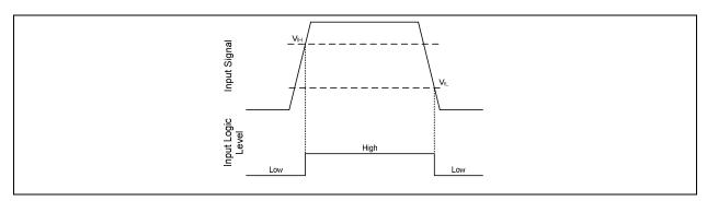
Figure 10 HIN & LIN input thresholds
