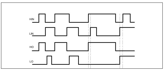
Figure 7 Ideal Input/output timing diagram
