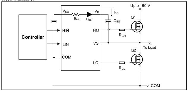
Figure 14 Half bridge bootstrap circuit in 2ED2744S01G
