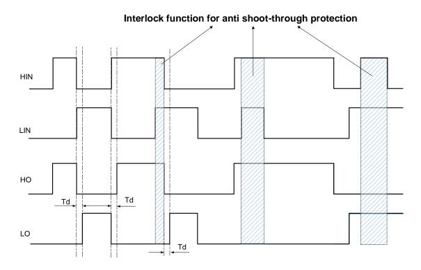
Figure 4 Input/output logic diagram
