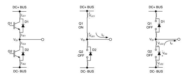
Figure 10 Parasitic Elements
