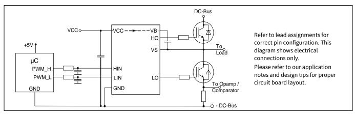
Figure 1 Typical application diagram
