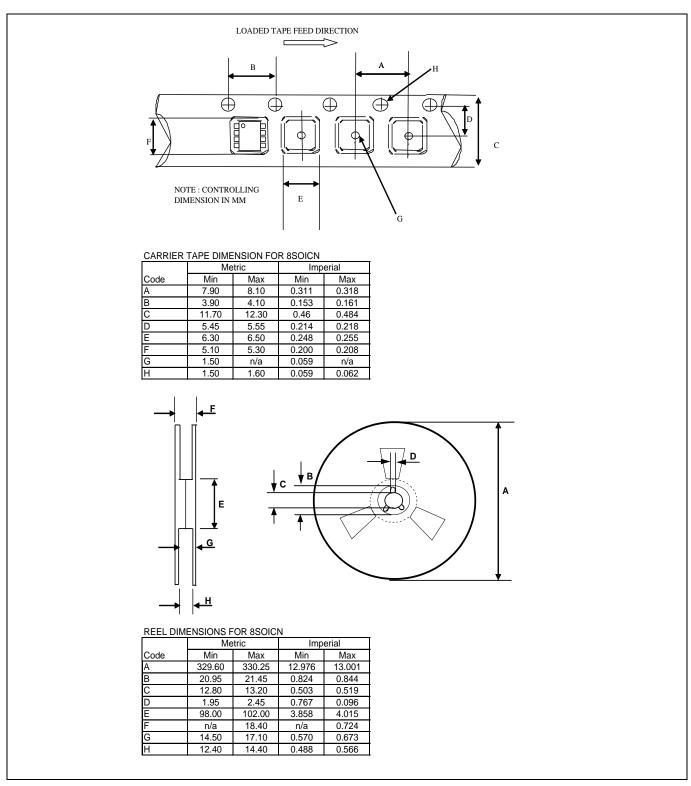
Figure 16 Tape and reel details PG-DSO-8
