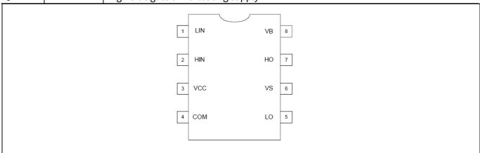
Figure 3 2ED2304S06F lead assignments PG-DSO-8 (top view)
