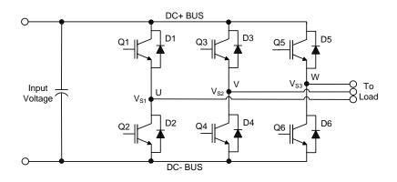
Figure 5 Three phase inverter
