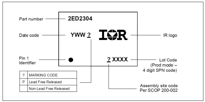
Figure 15 Marking information PG-DSO-8 (2ED2304S06F)
