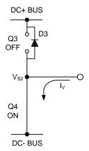
Figure 8 D3 conducting
