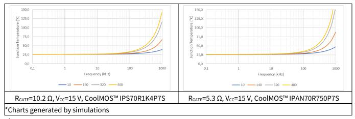
Figure 42 T<sub>J</sub> vs Frequency
