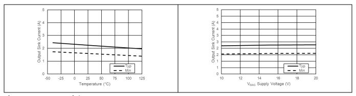
Figure 41 Output Sink Current
