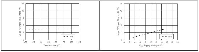
Figure 30 Logic "0" Input Threshold
