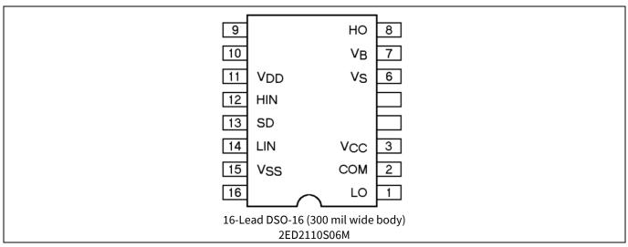
Figure 3 2ED2110S06M pin assignments (top view)
