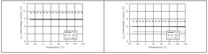
Figure 38 V<sub>BS</sub> Undervoltage Lockout
