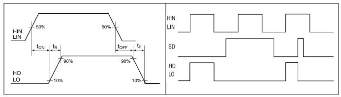
**Switching timing diagram** Figure 6
