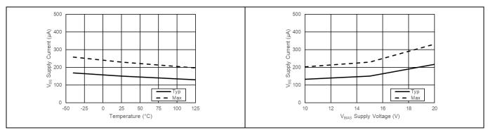
Figure 33 V<sub>BS</sub> Supply Current
