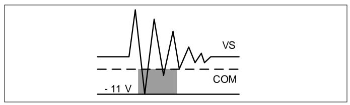
Figure 20 Headroom for HV level shifter data transmission
