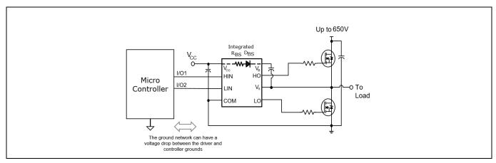
Figure 15 Negative voltage tolerance on inputs of up to -5 V
