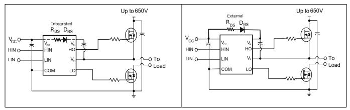
Figure 12 2ED2110S06M with integrated components
