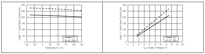
Figure 36 Logic "1" Input Bias Current
