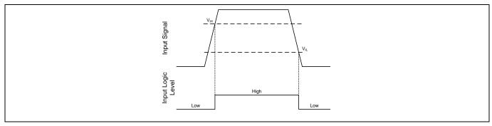
Figure 10 **HIN & LIN input thresholds**
