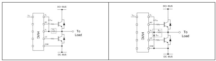
Figure 23 Resistor between the VS pin and the switch node and clamping diode between COM and Vs
