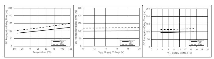
Figure 26 SD Propagation Delay Time
