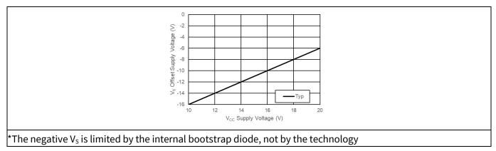
Figure 44 Negative V<sub>s</sub> vs V<sub>cc</sub>
