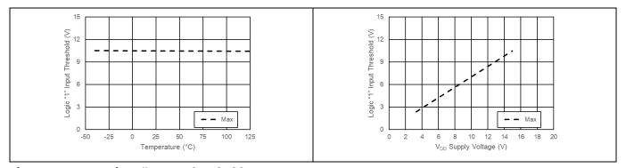
Figure 29 Logic "1" Input Threshold
