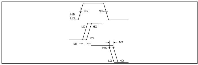
Figure 8 Delay matching waveform definition
