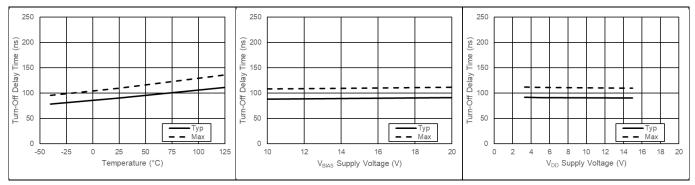
Figure 25 Turn-Off Delay Time
