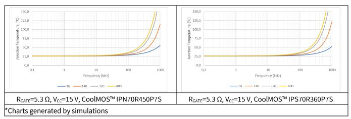
Figure 43 T<sub>J</sub> vs Frequency
