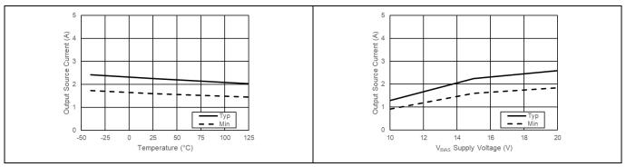
Figure 40 Output Source Current
