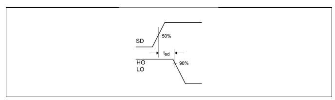
Figure 9 Shutdown waveform definitions
