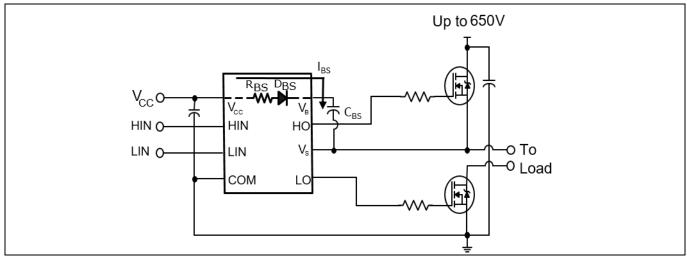
Figure 14 Half bridge bootstrap circuit in 2ED2110S06M
