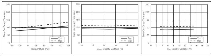
Figure 24 Turn-On Delay Time
