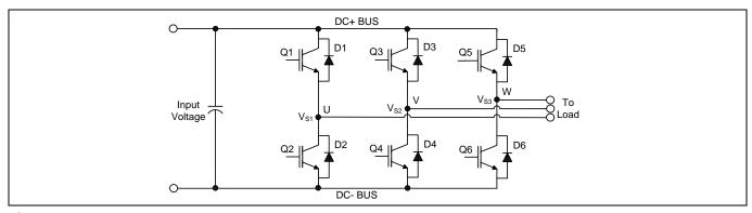
Figure 16 Three phase inverter
