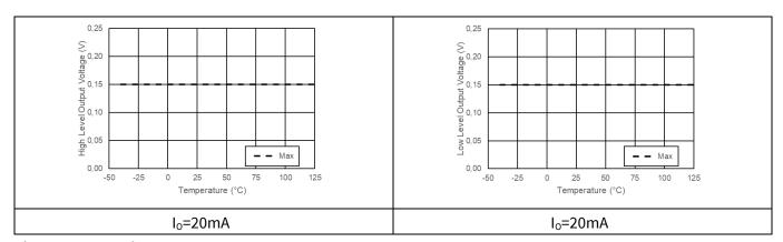
Figure 31 High/Low Level Output Voltage
