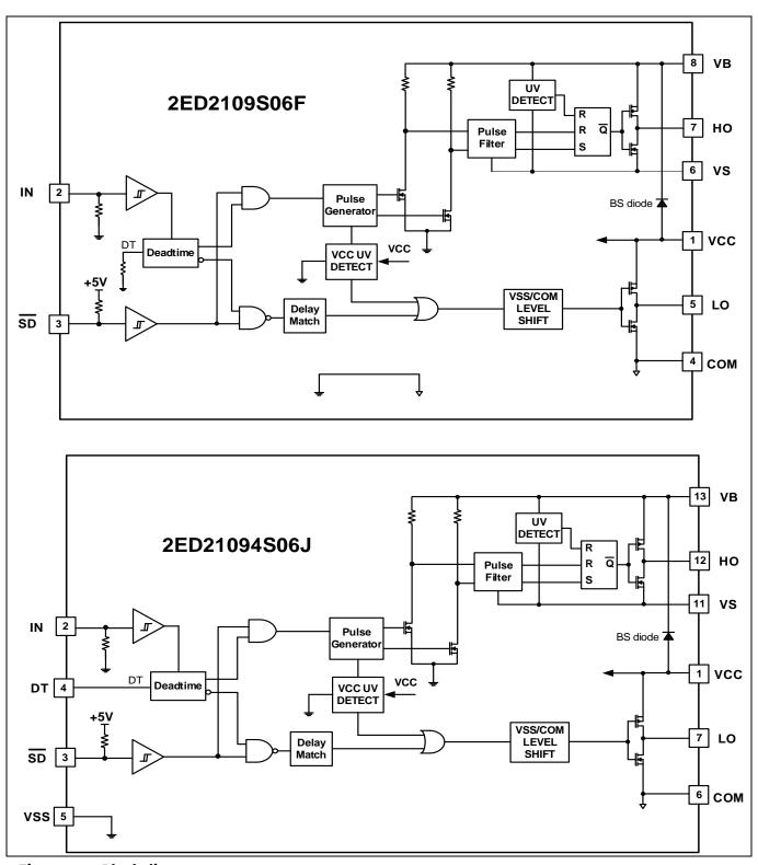
Figure 2 Block diagrams
