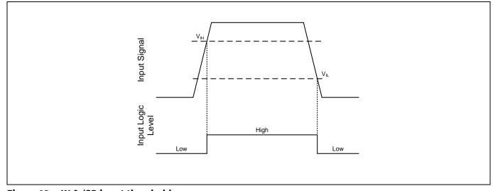
Figure 13 IN & /SD input thresholds
