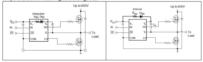
Figure 15 2ED210x with integrated components
