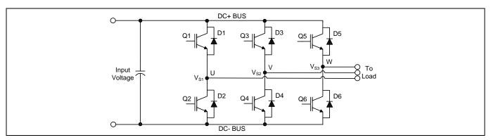
Figure 19 Three phase inverter
