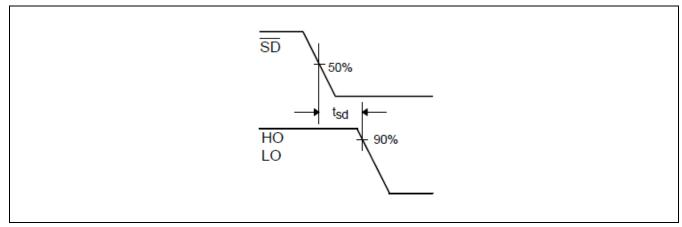
Figure 12 Shutdown waveform definitions
