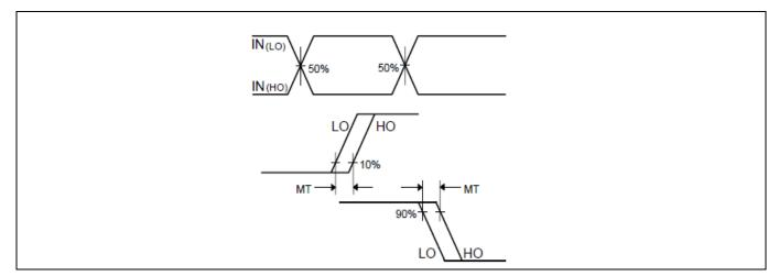
Figure 11 Deadtime matching waveform definition
