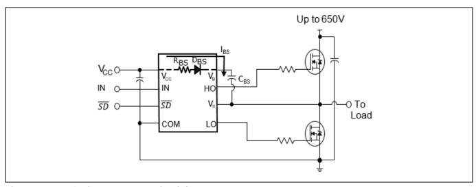
Figure 17 Half bridge bootstrap circuit in 2ED210x
