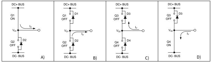
Figure 20 A) Q1 conducting
