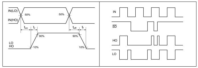
Figure 6 Switching timing diagram
