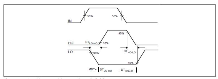
Figure 8 Deadtime matching waveform definition
